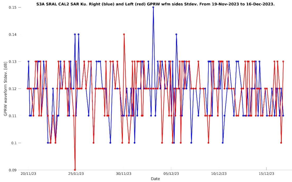
Figure 4-23. S3A CAL2 SAR Ku waveforms right (blue) and left (red) sides Standard Deviation over the period.
