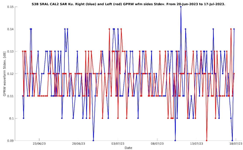
Figure 4-24. S3B CAL2 SAR Ku waveforms right (blue) and left (red) sides Standard Deviation over the period.
