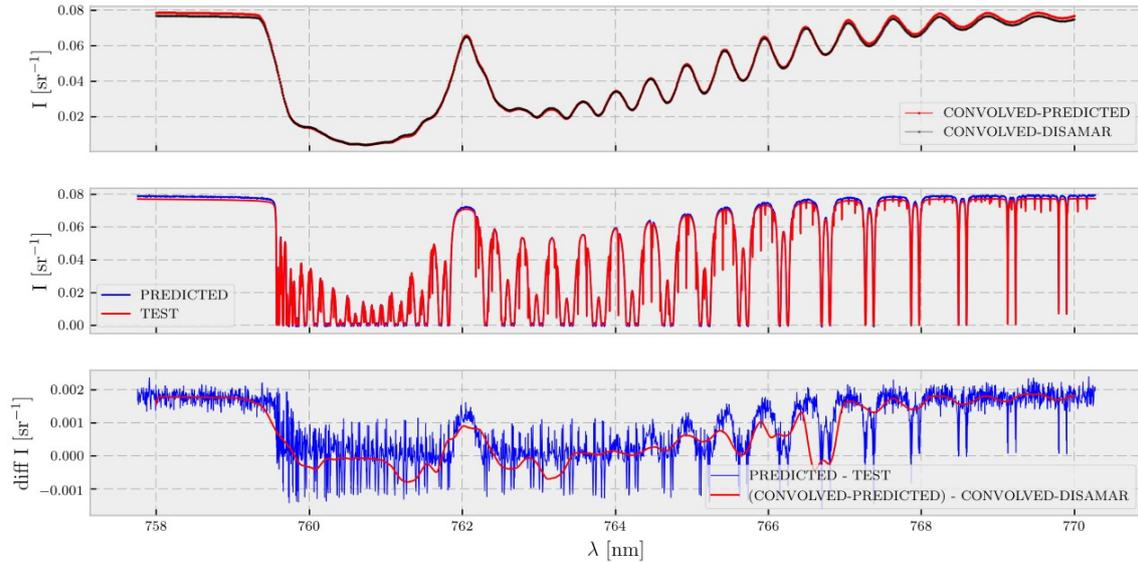
**Figure 8:** Example of the Sun-normalised radiance spectrum in the Oxygen-A band as computed by the RTM and by the NN model. The top panel shows the spectra after convolution with the S5P slit function, the middle panel shows a comparison between the high resolution spectra, and the bottom show the difference between the LBL and NN spectra, for the high resolution and convolved spectra.
