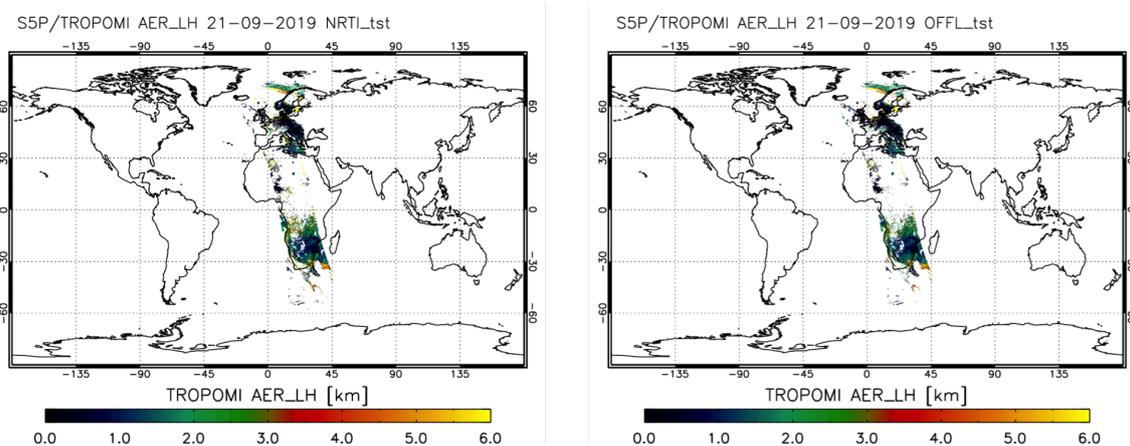
**Figure 5:** Difference in cloud masking between the NRTI processor (using FRESCO as a cloud mask) and the OFFL cloud processor (using VIIRS as a cloud mask).
