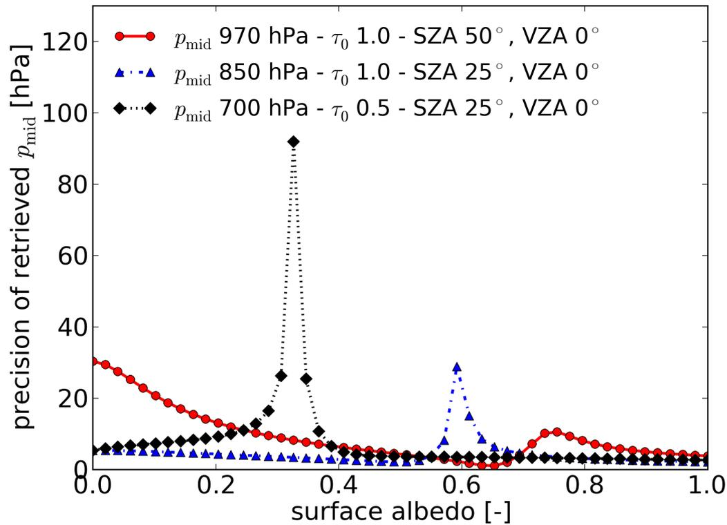
**Figure 19:** Precision of retrieved mid pressure as a function of surface albedo for three arbitrary atmospheric states and observation geometries.
