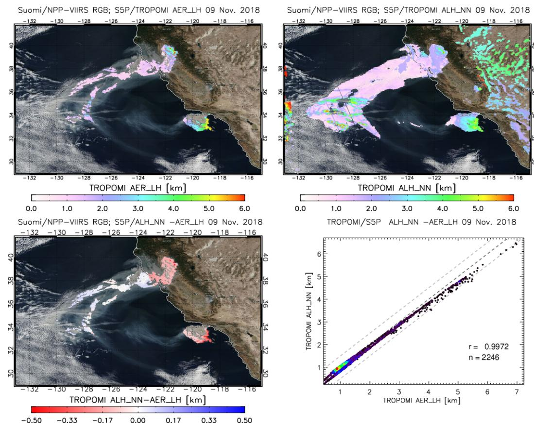
**Figure 13:** (top-left) Suomi/NPP VIIRS RGB on 9 Nov. 2018, overlaid with LBL ALH ; (top-right) Suomi/NPP VIIRS RGB on 9 Nov. 2018, overlaid with NN ALH; (bottom-left) Suomi/NPP VIIRS RGB on 9 Nov. 2018, overlaid with difference of NN-LBL ALH; (bottom-right) Scatterplot of NN ALH versus LBL ALH for the pixels in the left panels.
