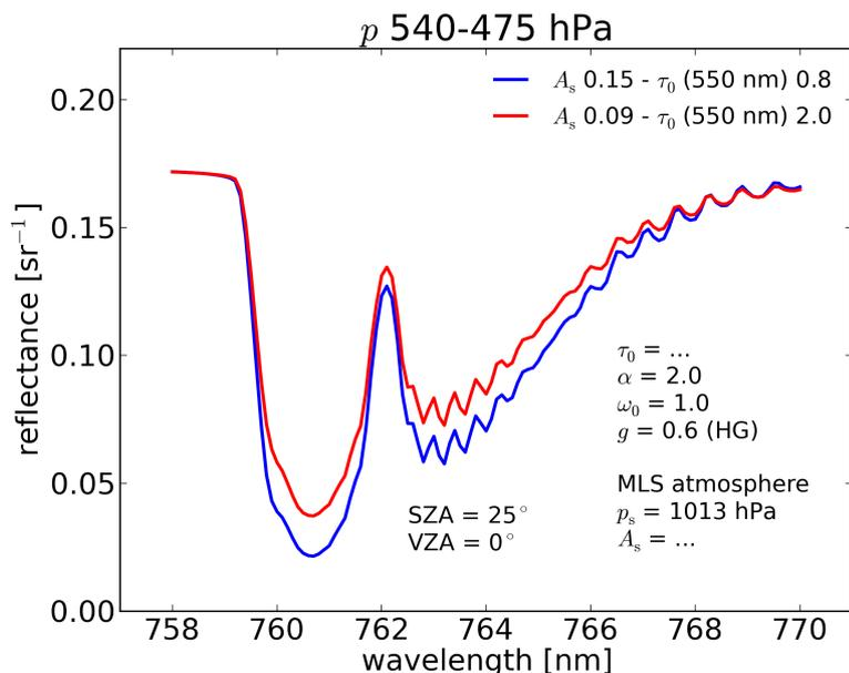
**Figure 24:** Reflectance spectra for two different combinations of optical thickness and surface albedo that yield the same continuum reflectance. All other parameters are the same. The aerosol layer is between 540 and 475 hPa; the single scattering albedo is 1.0; the solar zenith angle is 25° and the viewing direction is nadir. From the shape of absorption we can simultaneously fit surface albedo and aerosol optical thickness.
