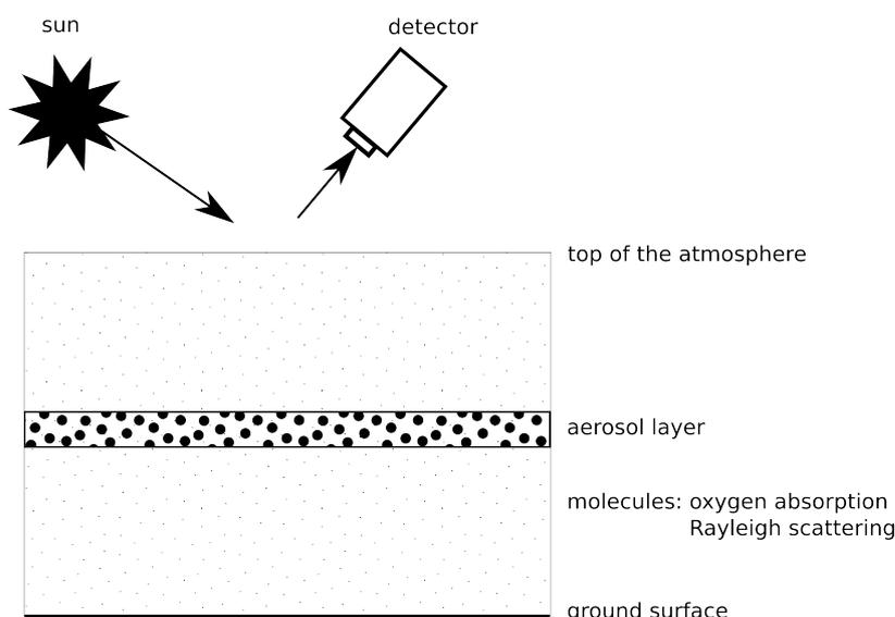
**Figure 2:** Schematic depiction of the atmosphere and typical TROPOMI satellite configuration for retrieval of Aerosol Layer Height. The Rayleigh scattering optical thickness at the O<sub>2</sub> A band is ~0.02
