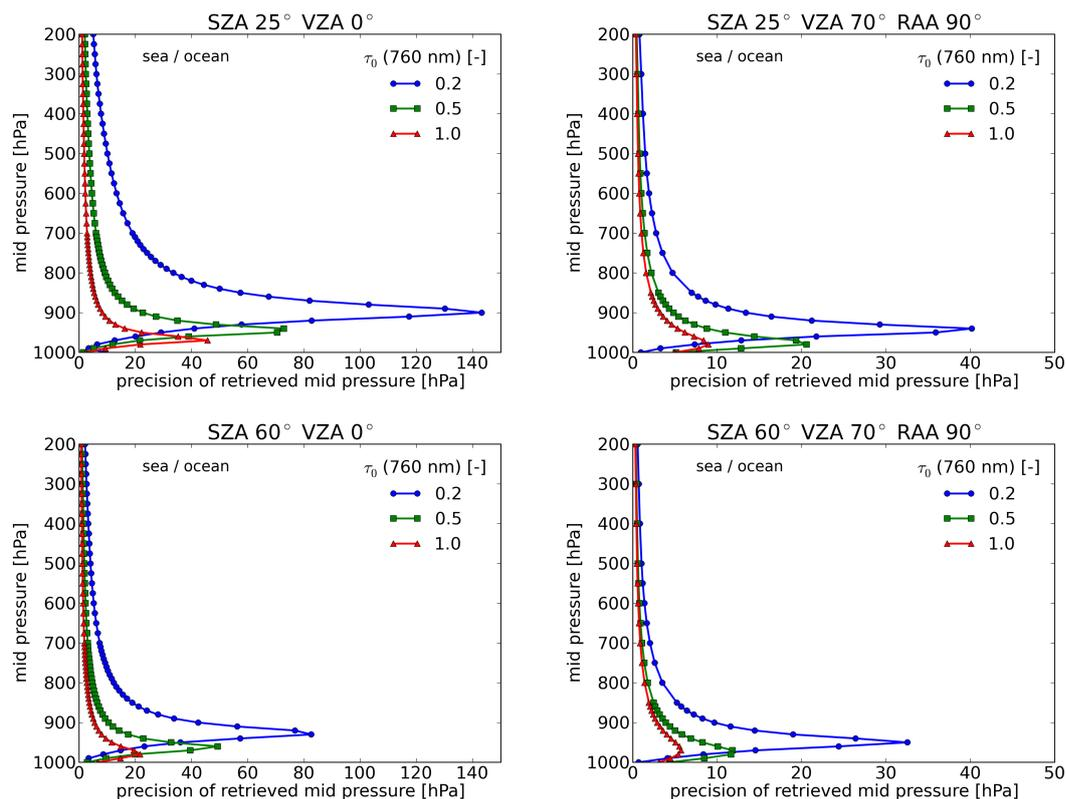
**Figure 17:** Precision of retrieved aerosol mid pressure as a function of mid pressure for three values of the aerosol optical thickness. Panel A shows retrieval precision for an aerosol layer over sea / ocean; Each of the four subplots in a panel corresponds to a different observation geometry: SZA 25°, VZA 0° (top left); SZA 25°, VZA 70°, RAA 90° (top right); SZA 60°, VZA 0° (bottom left); and SZA 60°, VZA 70°, RAA 90° (bottom right). Note the different scales of the x-axis.
