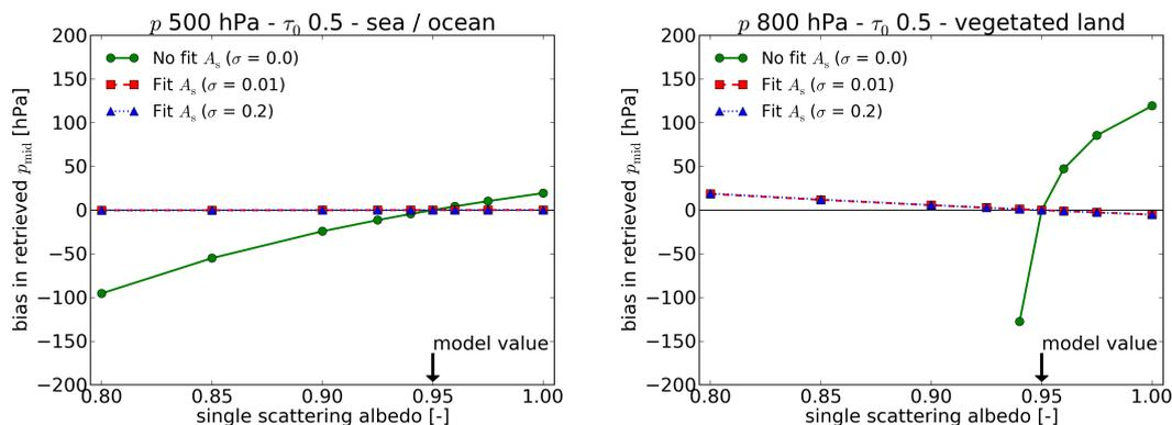
**Figure 26:** Effect of a model error in the single scattering albedo on the bias in retrieved pressure as a function of the true single scattering albedo for three retrieval types (Table 13). The single scattering albedo assumed in retrieval is 0.95. Left: aerosol layer with optical thickness of 0.5 at 500 hPa over sea / ocean; right: aerosol layer with optical thickness of 0.5 at 800 hPa over vegetated land. Missing data points indicate that retrieval does not converge.
