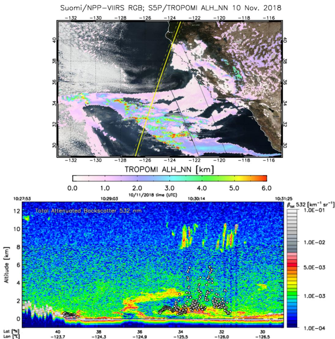
**Figure 32:** (top) Suomi/NPP VIIRS RGB on 10 Nov. 2018, overlaid with NN ALH. The yellow line depicts the CALIPSO track overpassing that day. The yellow dashed line depict the 20 km range around the CALIPSO track; (bottom) CALIP Total attenuated backscatter at 532 nm on 10 Nov. 2018 for the track shown by the yellow line in the top panel.
