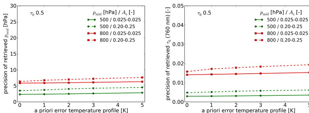
**Figure 27:** Precision of retrieved aerosol pressure (left plot) and optical thickness (right plot) as a function of the *a priori* error in the temperature profile. The aerosol layer has optical thickness of 0.5 and is located at 500 hPa (green lines) or 800 hPa (red lines), over sea / ocean (solid lines) or vegetated land (dashed lines). Retrieval precision shows the same behavior if the optical thickness is 0.2.
