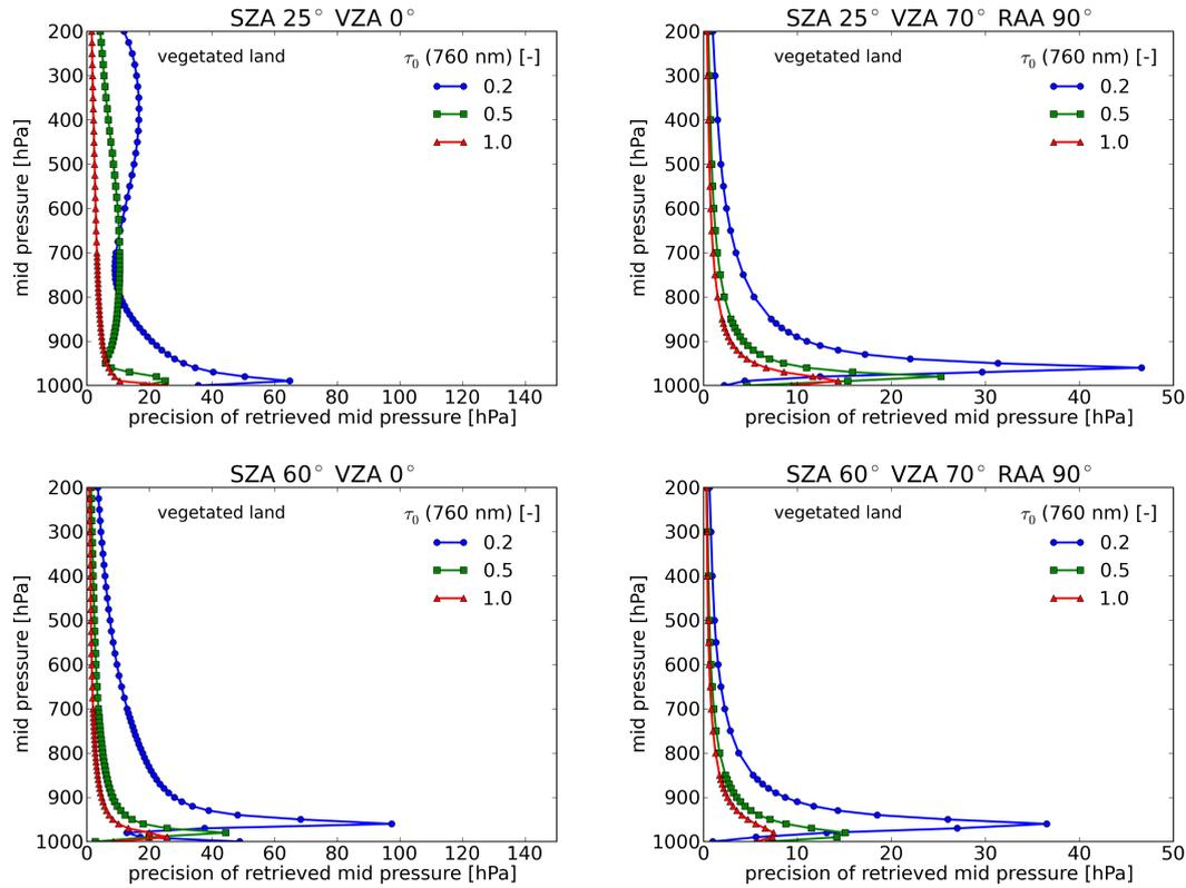
**Figure 18:** Precision of retrieved aerosol mid pressure as a function of mid pressure for three values of the aerosol optical thickness. Panel A shows retrieval precision for an aerosol layer over vegetated land. Each of the four subplots in a panel corresponds to a different observation geometry: SZA 25°, VZA 0° (top left); SZA 25°, VZA 70°, RAA 90° (top right); SZA 60°, VZA 0° (bottom left); and SZA 60°, VZA 70°, RAA 90° (bottom right). Note the different scales of the x-axis.
