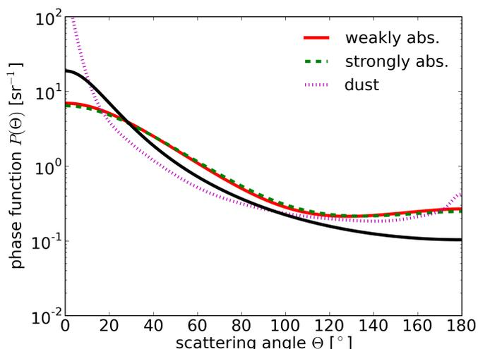
**Figure 22:** Phase functions for the three aerosol models used in the retrieval simulations of Figure 23. The black line corresponds to a Henyey-Greenstein phase function with asymmetry parameter of 0.7, which is used in retrieval.
