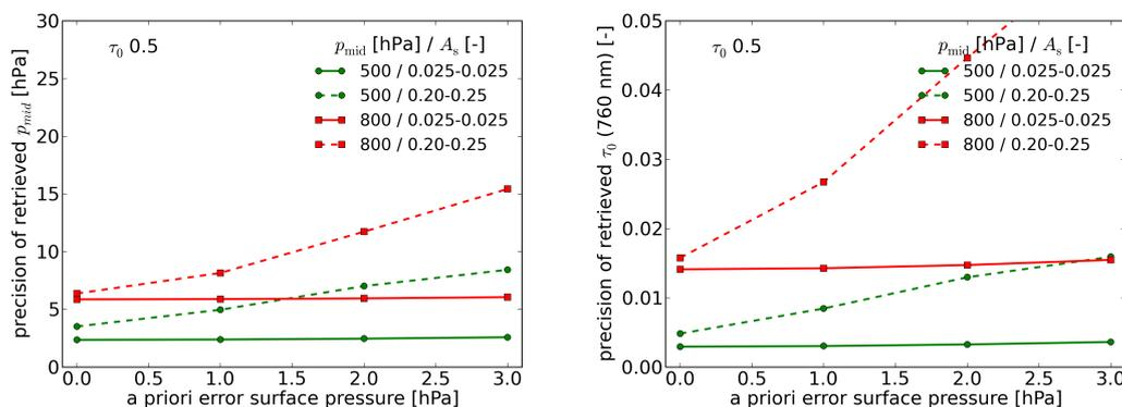
**Figure 28:** Precision of retrieved aerosol pressure (left plot) and optical thickness (right plot) as a function of the *a priori* error in the surface pressure. The aerosol layer has optical thickness of 0.5 and is located at 500 hPa (green lines) or 800 hPa (red lines), over sea / ocean (solid lines) or vegetated land (dashed lines). Retrieval precision shows the same behavior if the optical thickness is 0.2.
