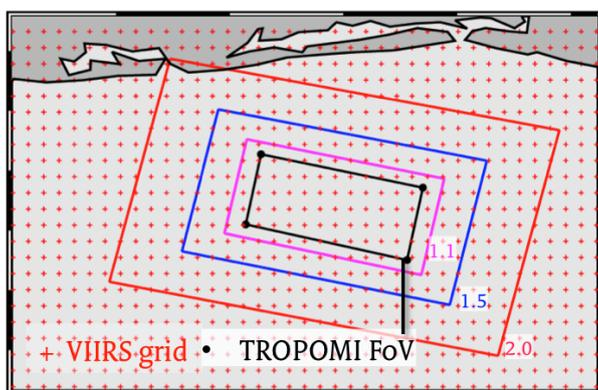
**Figure 6:** Schematic representation of the different Field-of-VIEWS (FoVs) as defined for the SNPP-VIIRS cloud mask for TROPOMI measurements. The smallest FoV (black) corresponds to the TROPOMI footprint with the corner point defined as the midpoints between the centers of the FoV. The others FoVs are larger (corresponding to 1.1, 1.5 and twice the amount of energy contained in the FoV), for users to increasingly filter more clouds, including those in neighbouring pixels.
