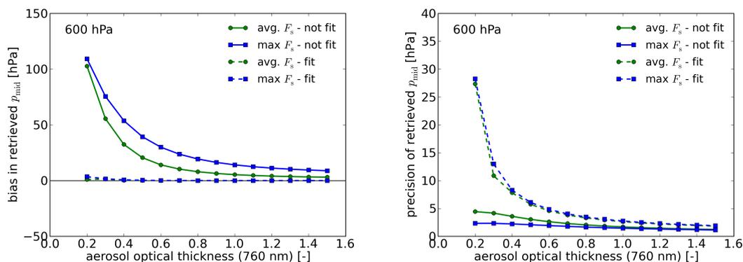
**Figure 31:** Accuracy (left plot) and precision (right plot) of retrieved aerosol pressure as a function of optical thickness when the vegetated land surface exhibits chlorophyll fluorescence. Solid lines correspond to a retrieval in which fluorescence is present in the simulation but not accounted for in the forward model for retrieval. Dashed lines correspond to a retrieval in which fluorescence emissions are included in the forward model and retrieved simultaneously with aerosol parameters.
