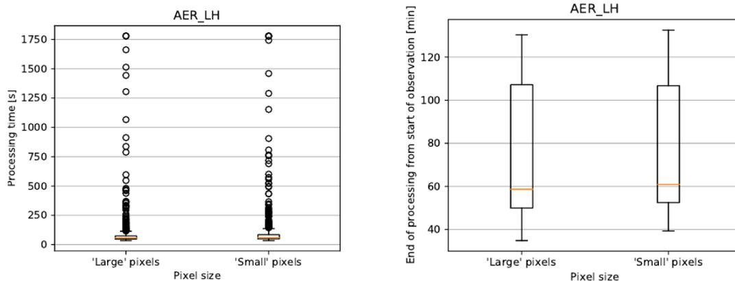
**Figure 11:** Timeliness of the AER\_LH processor. The upper panel shows the processing time per near-real time granule. The bottom panel shows the timeliness of the end of the processing time. ‘Large’ pixels refer to pixels with an integration time of 1080 ms, yielding pixel sizes of  $7 \times 7 \text{ km}^2$  at nadir, ‘small’ pixels refer to an integration time of 840 ms, yielding pixel sizes of about  $7 \times 5.6 \text{ km}^2$ .
