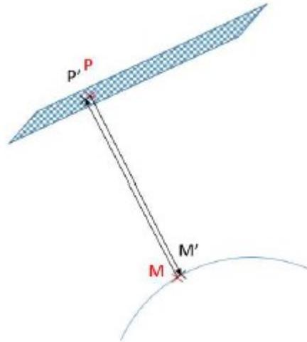
**Figure 15. Illustration of residuals distance values (P-P') and (M-M')**
