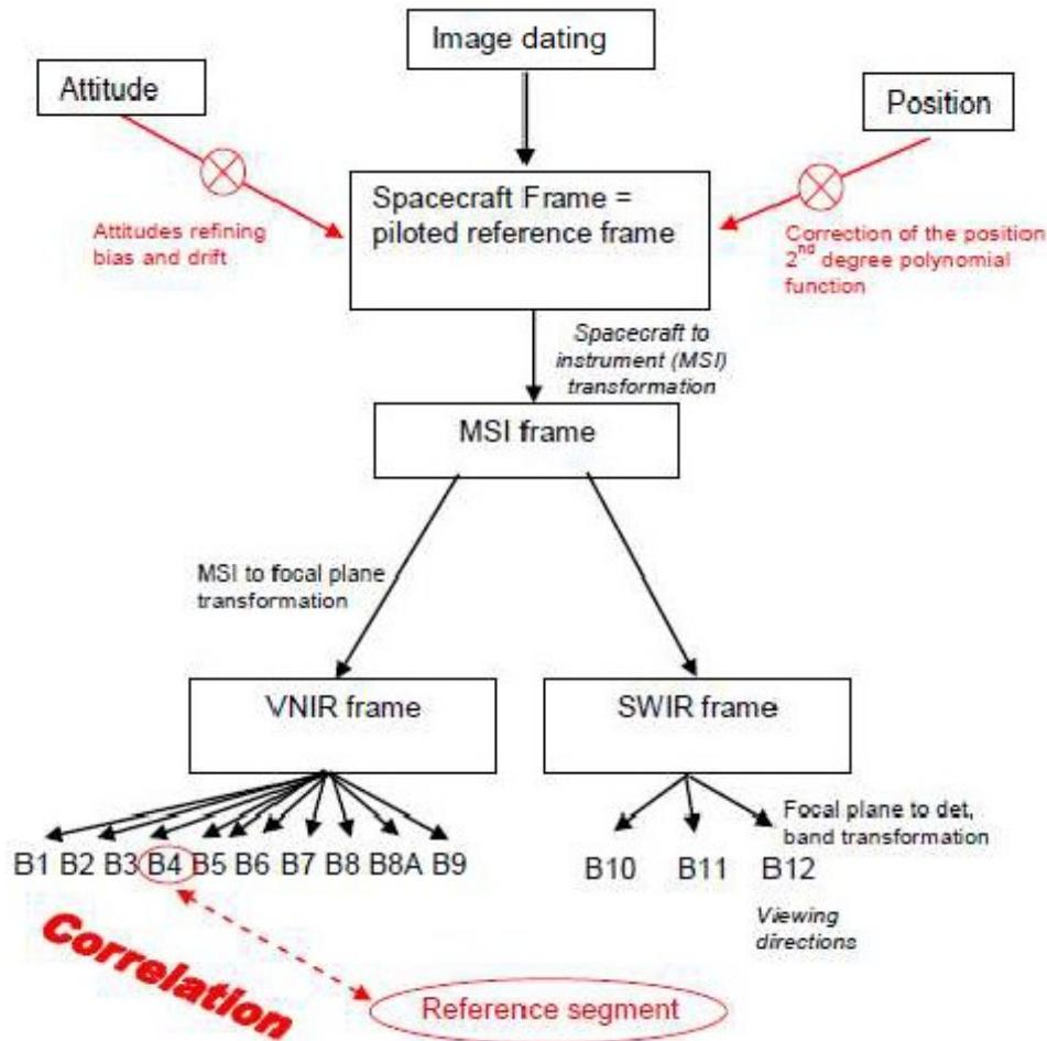
Figure 18. Viewing model and parameters to refine.
