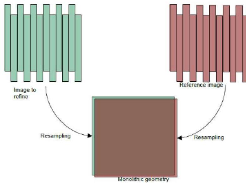
**Figure 16. Resampling in monolithic geometry.**
