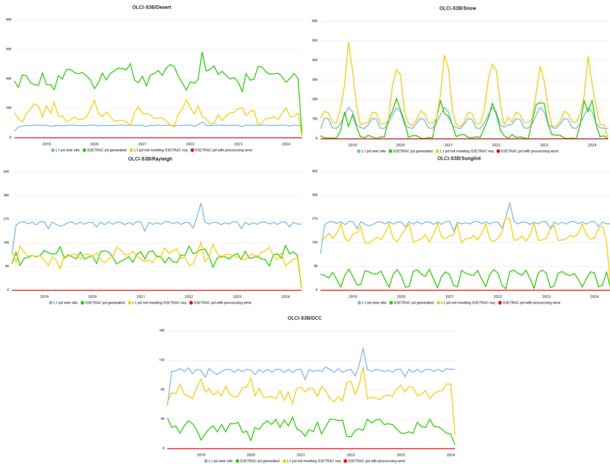
Figure 61: summary of S3ETRAC products generation for OLCI-B (number of OLCI-B L1 products Ingested, blue – number of S3ETRAC extracted products generated, green – number of S3ETRAC runs without generation of output product (data not meeting selection requirements), yellow – number of runs ending in error, red, one plot per site type).
