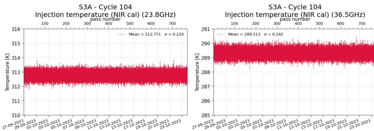
Figure 6 : Monitoring of S3A Noise Injection temperature for both channels :23.8GHz (left) and 36.5GHz (right)
