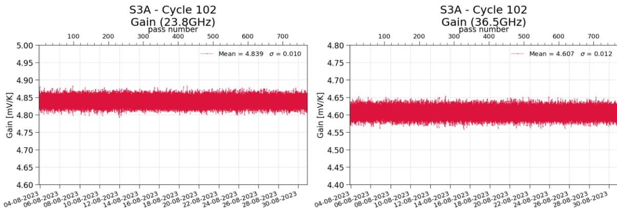
Figure 4 : S3A Monitoring of receiver gain for both channels :23.8GHz (left) and 36.5GHz (right)
