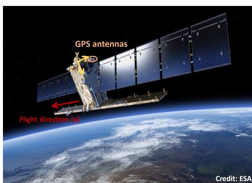
Figure 1: Artificial view of the Sentinel-1 satellite with the GPS antennas on top and axes in satellite bodyfixed reference system.
