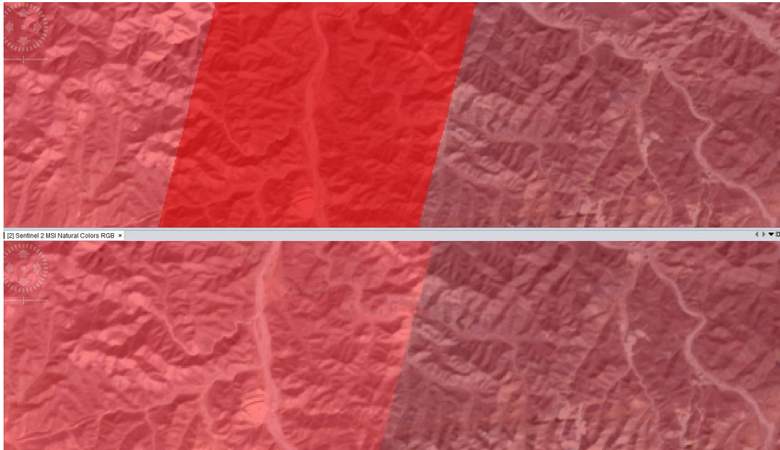
Figure 8: Detector footprints for the current processing baseline 02.06 (top) and new processing baseline 02.07 (bottom). The detector footprint does no longer include the overlap area.
