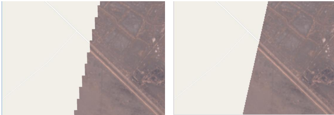
Figure 7: Swath boundary with the processing baseline 02.06 (Left) and new processing baseline 02.07 (Right). The coarse staircase-like boundary has been refined. More valid pixels are provided.
