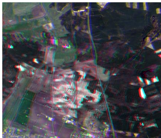
Figure 14: Spectral co-registration error (anomaly #14).
