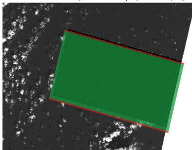
Figure 18: Technical Quality masks (green: lost packets, red: degraded packets) overlayed over an affected image. A small gap exists between the mask and the affected area (anomaly #24).
