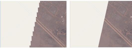
Figure 7: Swath boundary with the processing baseline 02.06 (Left) and new processing baseline 02.07 (Right). The coarse staircase-like boundary has been refined. More valid pixels are provided.
