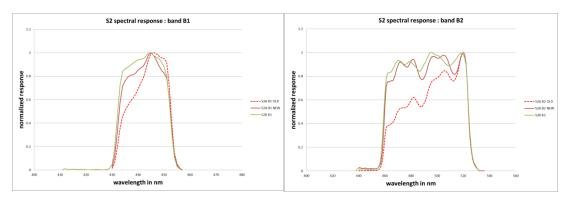
Figure 19: Spectral Response Functions for bands B01 and B02. Red – dashed: S2A before correction. Red – solid: S2A after correction. Green: S2B.
