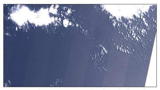
Figure 27: Stripe pattern over sea surface, due to the observation parallax effect between odd and even detectors.
