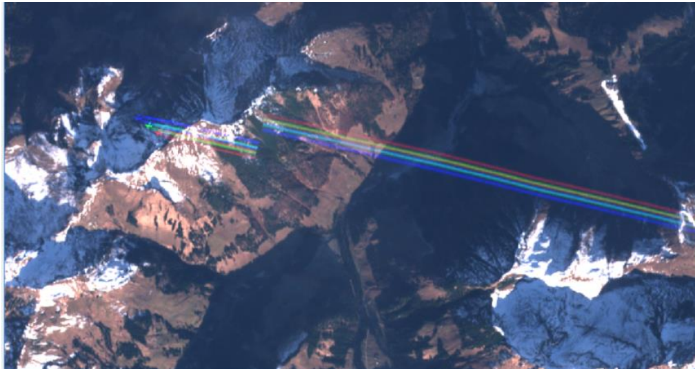
Figure 28: Spectral misregistration and detector misalignment for object at high altitude (plane and contrail). This feature is not an anomaly.
