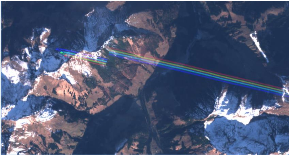
Figure 28: Spectral misregistration and detector misalignment for object at high altitude (plane and contrail). This feature is not an anomaly.
