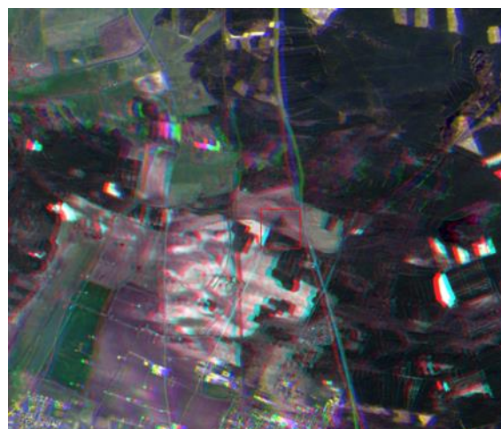
Figure 14: Spectral co-registration error (anomaly #14).
