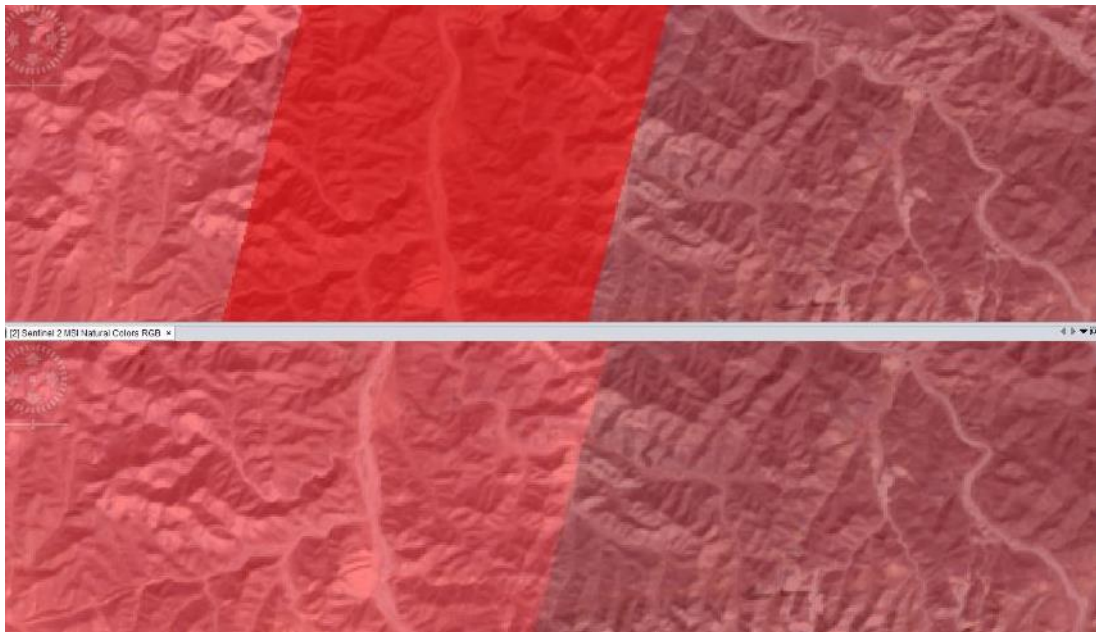
Figure 8: Detector footprints for the current processing baseline 02.06 (top) and new processing baseline 02.07 (bottom). The detector footprint longer includes the overlap area.
