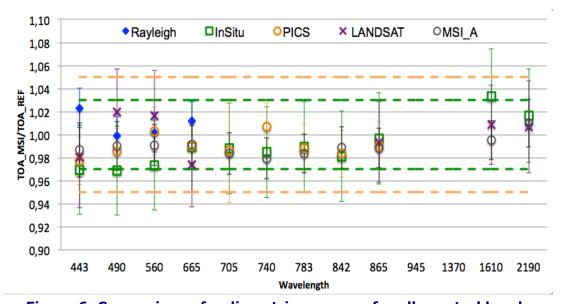
Figure 6: Comparison of radiometric accuracy for all spectral bands (except B09 & B10): ratio of S2B measurement on reference. Error bars indicate the method uncertainty. 06/2021
