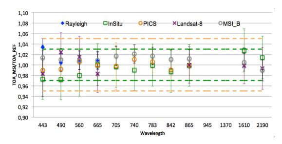
Figure 5: Comparison of radiometric accuracy for all spectral bands (except B09 and B10): ratio of S2A measurement on reference. Error bars indicate the method uncertainty. 06/2021
