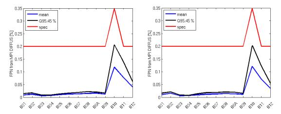
Figure 8: Fixed Pattern Noise (residual error after equalization) measured on diffuser images for S2A (left) and S2B (right). Blue curve: mean FPN, black: 95 percentile, red: specified value.
