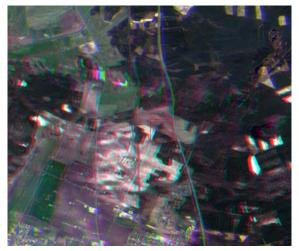
Figure 14: Spectral co-registration error (anomaly #14).
