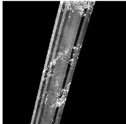
**Figure 22: Incorrect equalization of B10 for S2A (anomaly #45).**
