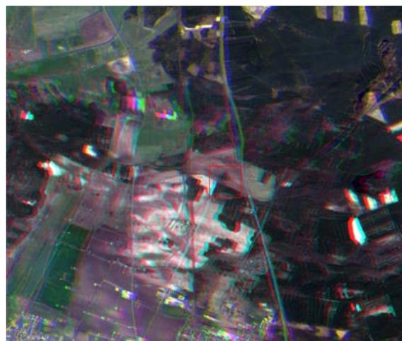
**Figure 14: Spectral co-registration error (anomaly #14).**
