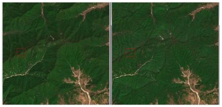
Figure 4-4: Left: affected product processed without DEM. Right: corrected product processed with DEM (anomaly #7).
