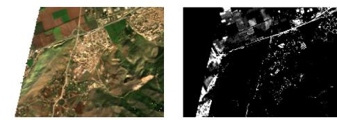
Figure 4-3: incorrect values of the cloud probability mask (CLDPRB) near the boundary of the swath. Left: L2A true colour image, Right: CLDPRB mask.
