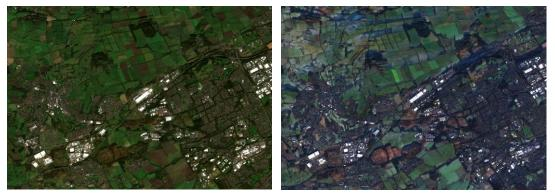
Figure 5-4: L2A True Colour Image of tile 30VVH; left: 10/10/2018, SZA = 62°; right: 24/12/208, SZA = 80°. The radiometric quality for surface reflectance is not ensured for SZA > 70°.
