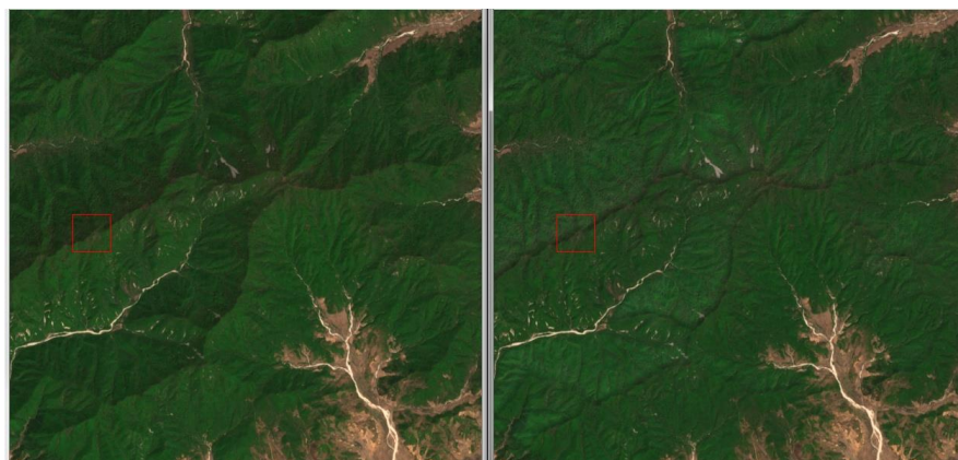
Figure 4-4: Left: affected product processed without DEM. Right: corrected product processed with DEM (anomaly #7).
