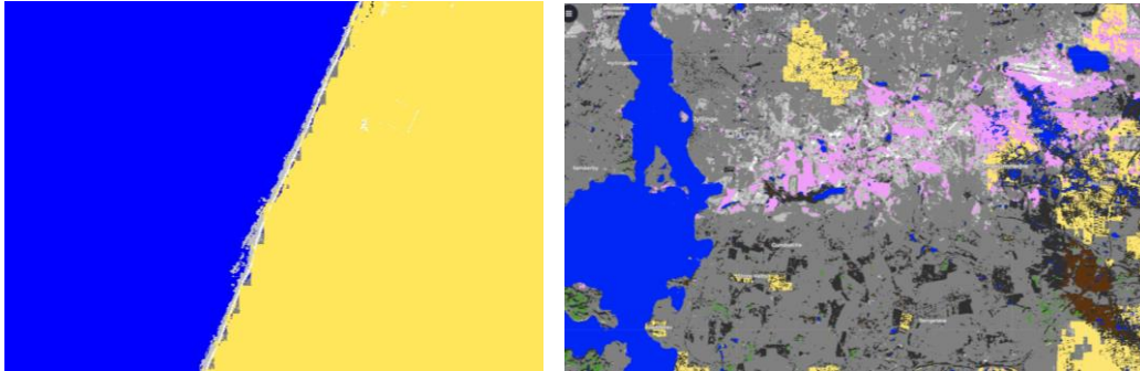
Figure 5-2: Blocky patterns on the scene classification layer (SCL). Left: near the coastline. Right: near city boundaries.
