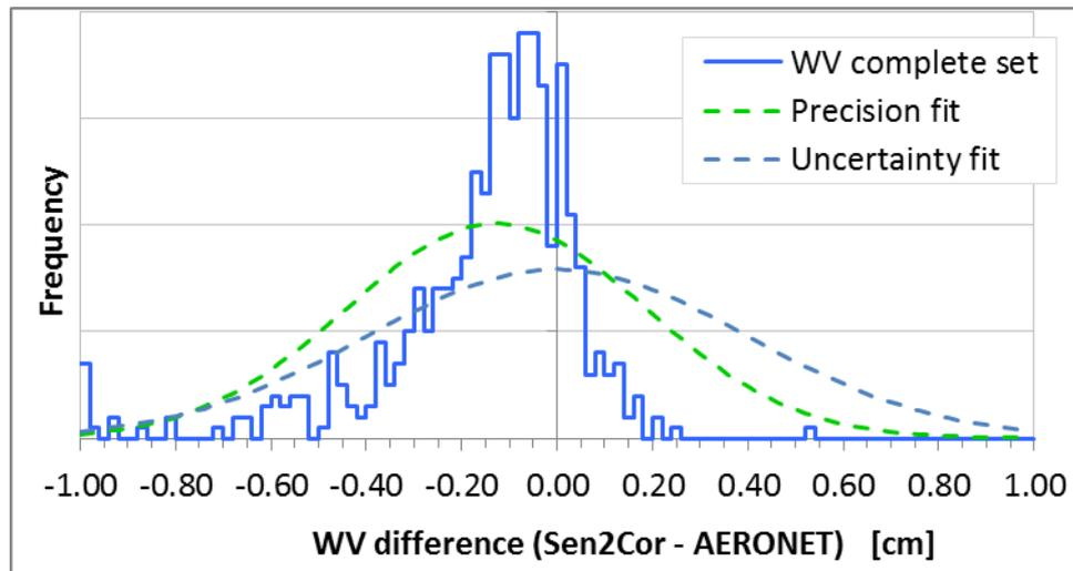
**Figure 2-4: Histogram plot of WV (at 20 m resolution) retrieval difference to the reference value from AERONET.** The green dashed curve gives a normal distribution computed with accuracy as mean value and precision as standard deviation. The blue dashed curve represents a normal distribution around zero with uncertainty as standard deviation.
