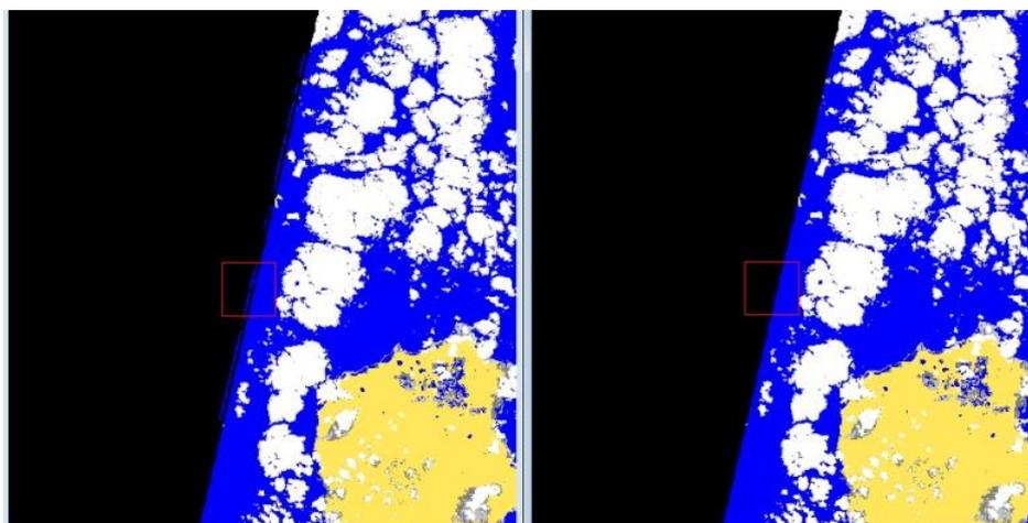
**Figure 4-1: Incorrect No Data Mask (anomaly #2).** Left: pixels incorrectly flagged as water (blue) near the swath edge. Right: same image after correction.
