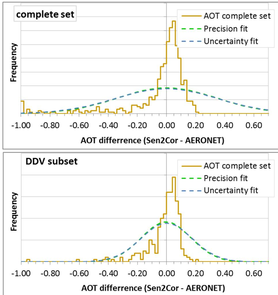
**Figure 2-6: Histogram plots of AOT<sub>550</sub> (at 20 m resolution) retrieval difference to the reference value from AERONET.** The blue dashed curves give normal distributions around zero with uncertainty as standard deviation. The upper plot shows results for the complete data set and the lower plot for the subset of images containing more than 2% DDV-pixels.
