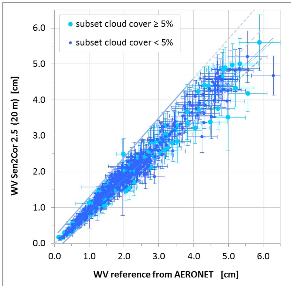
**Figure 2-3: Correlation plot of Sen2Cor WV retrieval at 20 m resolution over WV reference from AERONET on basis of a data set at 25 AERONET sites.** The dashed line indicates  $x=y$  and the solid lines show the limits of uncertainty requirement  $|\Delta WV| \leq 0.1 * WV_{ref} + 0.2$ .
