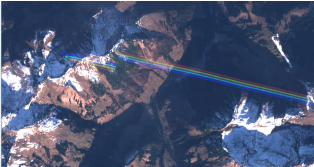
Figure 30: Spectral misregistration and detector misalignment for object at high altitude (plane and contrail). This feature is not an anomaly.
