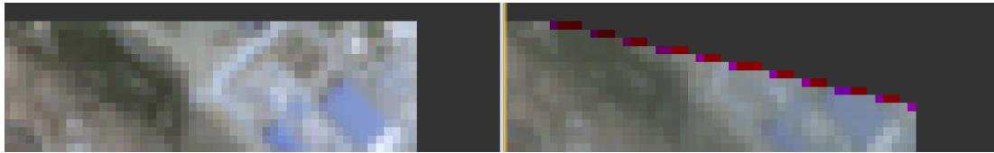
Figure 25: Top-right corner of the image of the same L1C tile from orbit 7053 (unaffected, left) and orbit 7196 (affected, right). (Anomaly #46)
