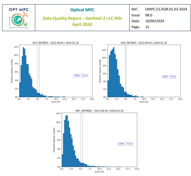
Figure 10: Multi-temporal 2D co-registration errors for refined S2A (upper left) and S2B pairs (upper right), and all pairs (bottom). The 95.45% performance is around 5 m.
