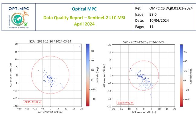
Figure 5: Relative geolocation performance for unrefined products. Left: S2A, Right: S2B.
