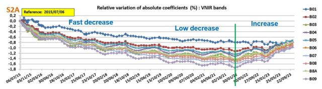
Figure 1: Relative variation of the absolute gain coefficients for VNIR bands of MSI-A, with respect to the first Sun acquisition on 6<sup>th</sup> of July 2015.
