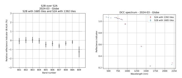
Figure 14 : DCC inter-calibration ratio between S2A and S2B as a function of the band number (left); DCC reflectance indicator for S2A and S2B as a function of the wavelength (right) assessed based on acquisitions from March 2024, on the globe. Reflectance indicator for all wavebands in the VNIR shows an alignment of S2A compared to S2B following the introduction of the radiometric harmonization factor on 01/2022.
