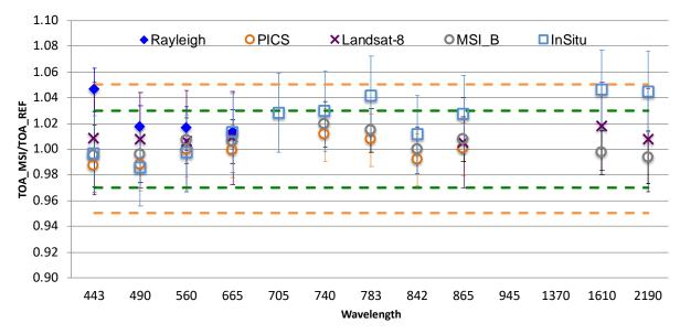
Figure 12: Comparison of radiometric accuracy for all spectral bands (except B09 and B10): ratio of S2A measurement on reference (top) pre-radiometric harmonization between Sentinel-2A and Sentinel-2B in January 2022, (bottom) post-radiometric harmonization up to 12/2023. Error bars indicate the method uncertainty.
