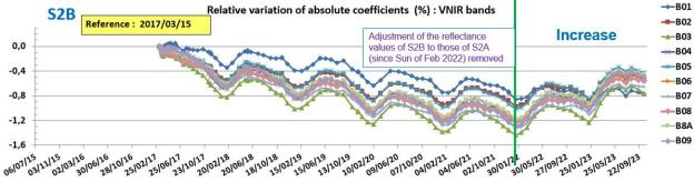
Figure 2: Relative variation of the absolute gain coefficients for VNIR bands of MSI-B, with respect to the first Sun acquisition on 15<sup>th</sup> of March 2017. The radiometric harmonization (applied since 25<sup>th</sup> January 2022) has been removed from this time series to make clearly noticeable the time variation of absolute gains.
