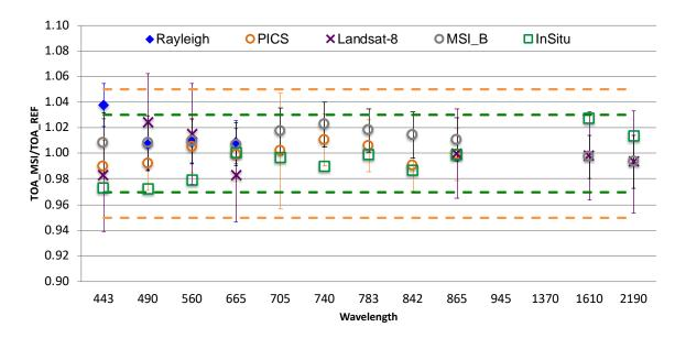
All results are within the 5% (3%) radiometric accuracy requirement (Goal) respectively.
