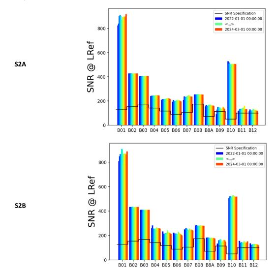
Figure 16 : Evolution of the SNR performances based on homogeneous natural acquisitions for S2A (top) and S2B (bottom) from 01/02/2022 to 31/02/2024
