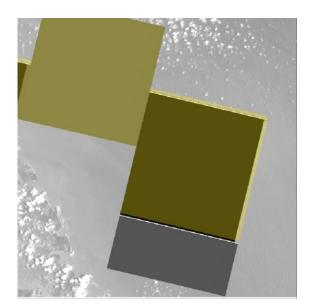
Figure 21: B02 of S2B\_MSIL1C\_20230110T073159\_N0509\_R049\_T36KYC\_20230110T092744 in background with band 3 (dedicated to lost packets) of the corresponding MSK\_QUALIT superimposed in yellow. All the black pixels, due to data loss, in B02 are not flagged in the quality mask.
