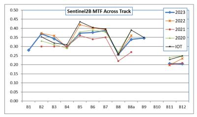
*Figure 20 : MTF performance assessments for S2B (along and across track) performed using products from last 4 years and compared to IOT measurements.*
