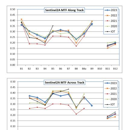
Figure 19 : MTF performance assessments for S2A (along and across track) performed using products from last 4 years and compared to IOT measurements.
