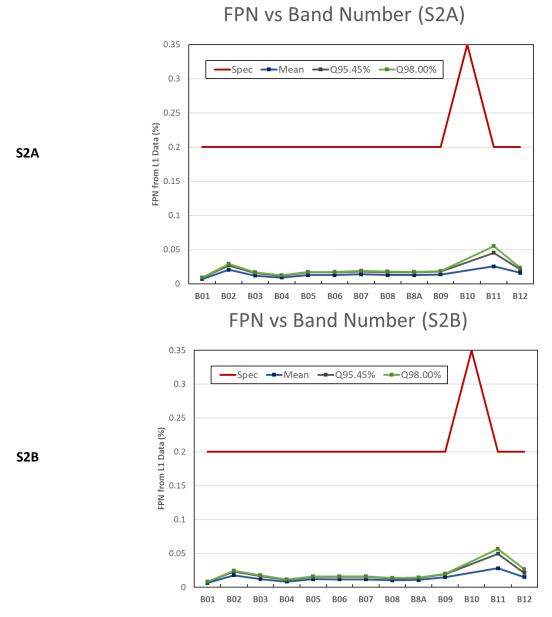
Figure 18 : Fixed Pattern Noise (residual error after equalization) measured on homogeneous natural images for S2A (left) and S2B (right) for February 2024.
