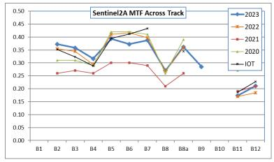
Figure 19: MTF performance assessments for S2A (along and across track) performed using products from last 4 years and compared to IOT measurements.
