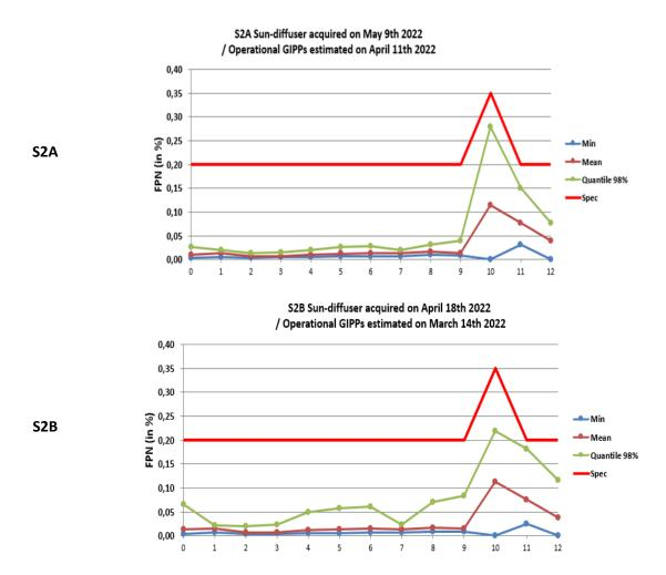
Figure 17: Fixed Pattern Noise (residual error after equalization) measured on diffuser images for S2A (top) and S2B (bottom). Blue curve: min FPN, marron: mean, green: 98 percentile, red: specified value.
