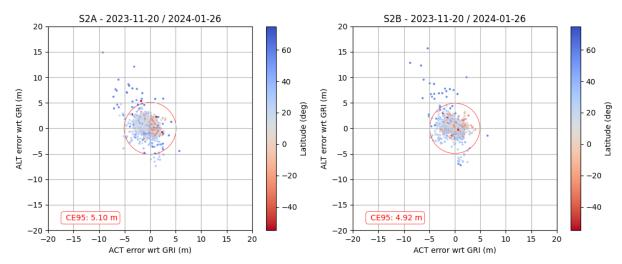
Figure 6: Relative geolocation performance for refined products. Left: S2A, Right: S2B
