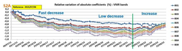
Figure 1: Relative variation of the absolute gain coefficients for VNIR bands of MSI-A, with respect to the first Sun acquisition on 6<sup>th</sup> of July 2015.
