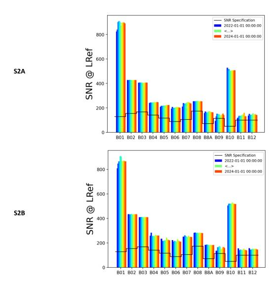
Figure 16 : Evolution of the SNR performances based on homogeneous natural acquisitions for S2A (top) and S2B (bottom) from 01/01/2022 to 01/12/2023
