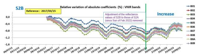
Figure 2: Relative variation of the absolute gain coefficients for VNIR bands of MSI-B, with respect to the first Sun acquisition on 15<sup>th</sup> of March 2017. The radiometric harmonization (applied since 25<sup>th</sup> January 2022) has been removed from this time series to make clearly noticeable the time variation of absolute gains.
