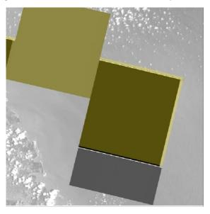
Figure 22: B02 of S2B\_MSIL1C\_20230110T073159\_N0509\_R049\_T36KYC\_20230110T092744 in background with band 3 (dedicated to lost packets) of the corresponding MSK\_QUALIT superimposed in yellow. All the black pixels, due to data loss, in B02 are not flagged in the quality mask.
