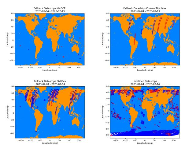
Figure 4 : Location of datastrips in fall-back and unrefined over a cycle period in February 2023 for S2A (red datastrips) and S2B (blue datastrips)
