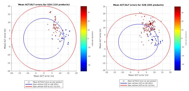
Figure 7: Absolute geolocation performance for unrefined products. Left: S2A, Right: S2B (01.2022 – 09.2023)
