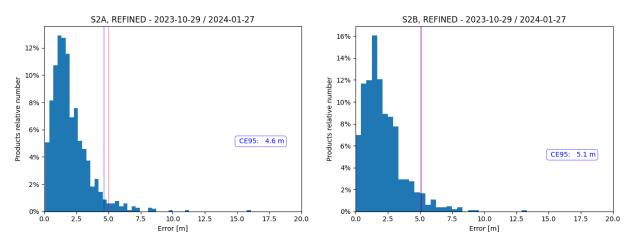
Figure 10: Multi-temporal 2D co-registration errors for refined S2A (left) and S2B pairs (right)
