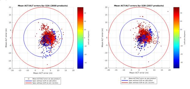
Figure 8: Absolute geolocation performance for refined products. Left: S2A, Right: S2B (01.2022 – 12.2023)
