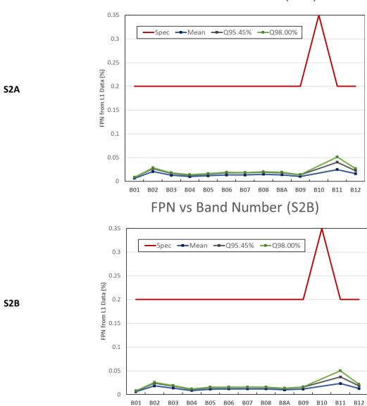
Figure 18 : Fixed Pattern Noise (residual error after equalization) measured on homogeneous natural images for S2A (left) and S2B (right) for September 2023.
