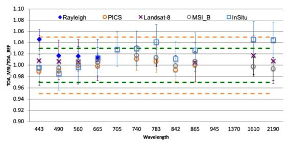
Figure 12: Comparison of radiometric accuracy for all spectral bands (except B09 and B10): ratio of S2A measurement on reference (top) pre-radiometric harmonization between Sentinel-2A and Sentinel-2B in January 2022, (bottom) post-radiometric harmonization up to 10/2023.
