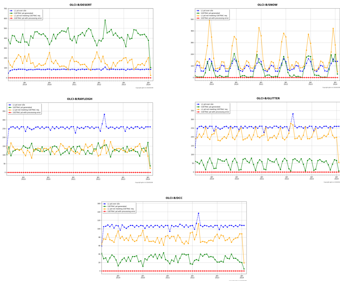
Figure 61: summary of S3ETRAC products generation for OLCI-B (number of OLCI-B L1 products Ingested, yellow – number of S3ETRAC extracted products generated, blue – number of S3ETRAC runs without generation of output product (data not meeting selection requirements), green – number of runs ending in error, red, one plot per site type).
