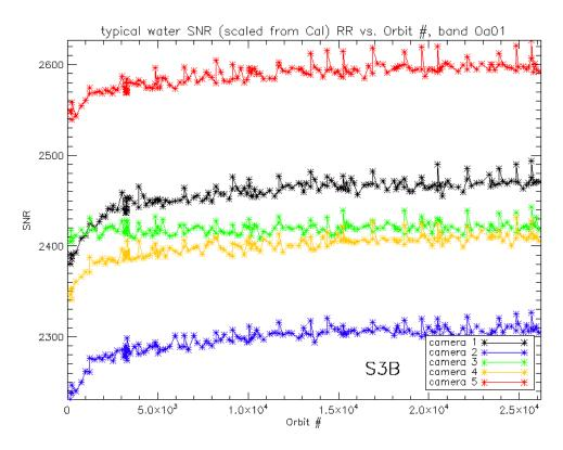
*Figure 43: long-term stability of the OLCI-B SNR estimates from Calibration data, example of channel Oa1.*
