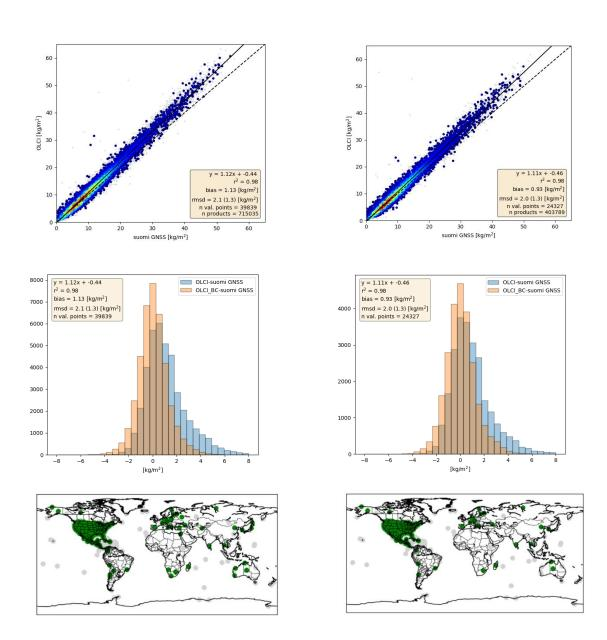
Figure 103: Upper: Scatter plot of the IWV products, derived from OLCI (A left, B right) above land and from SUOMI NET GNSS measurements. Middle: Histogram of the difference between OLCI (A: left, B: right) and GNSS (blue: original OLCI, orange: bias corrected OLCI). Lower: Positions of the GNSS (A: left, B: right).
