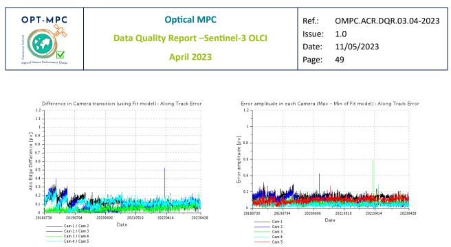
Figure 59: OLCI-B spatial along-track misregistration at each camera transition (left) and maximum amplitude of the along-track error within each camera (left).
