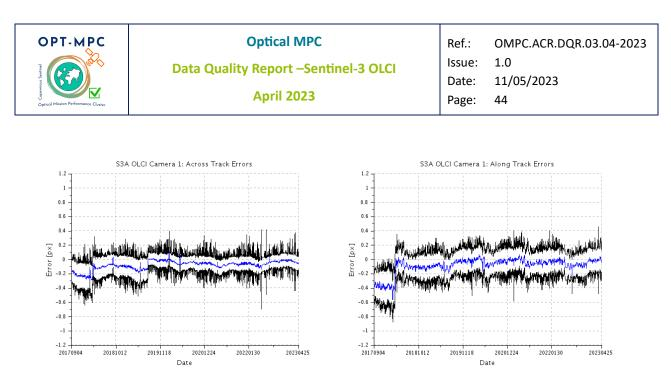
Figure 45: across-track (left) and along-track (right) OLCI-A georeferencing biases time series for Camera 1. Blue line is the average, black lines are average plus and minus 1 sigma.
