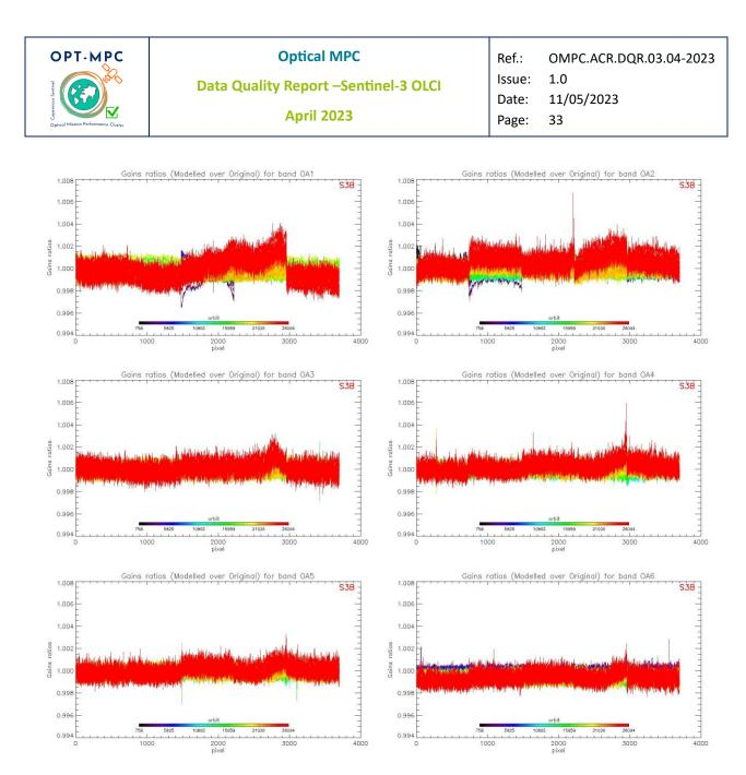
Figure 37: OLCI-B evolution model performance, as ratio of Model over Data vs. pixels, all cameras side by side, over the whole current calibration dataset (since instrument programming update), including 26 calibrations in extrapolation, channels Oa1 to Oa6.
