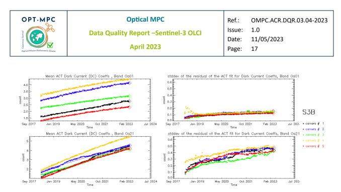
Figure 20: left column: ACT mean on 400 first detectors of OLCI-B Dark Current coefficients for spectral band Oa01 (top) and Oa21 (bottom). Right column: same as left column but for Standard deviation instead of mean. We see an increase of the DC level as a function of time especially for band Oa21.
