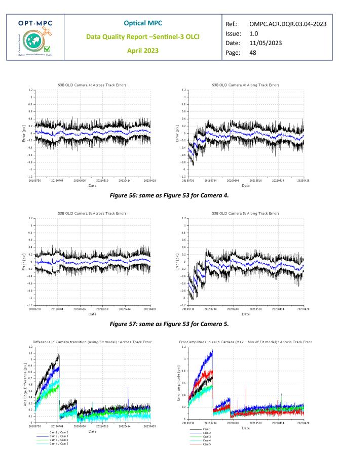
Figure 58: OLCI-B spatial across-track misregistration at each camera transition (left) and maximum amplitude of the across-track error within each camera (left).
