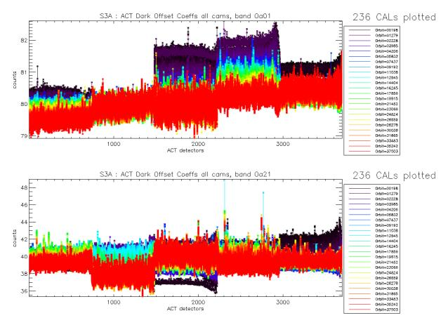
Figure 10: OLCI-A Dark Offset for band Oa1 (top) and Oa21 (bottom), all radiometric calibrations so far except the first one (orbit 183) for which the instrument was not thermally stable yet.
