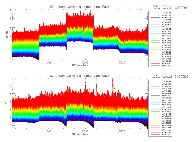
Figure 13: OLCI-A Dark Current for band Oa1 (top) and Oa21 (bottom), all radiometric calibrations so far except the first one (orbit 183) for which the instrument was not thermally stable yet.
