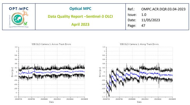
Figure 53: across-track (left) and along-track (right) OLCI-B georeferencing biases time series for Camera 1.
