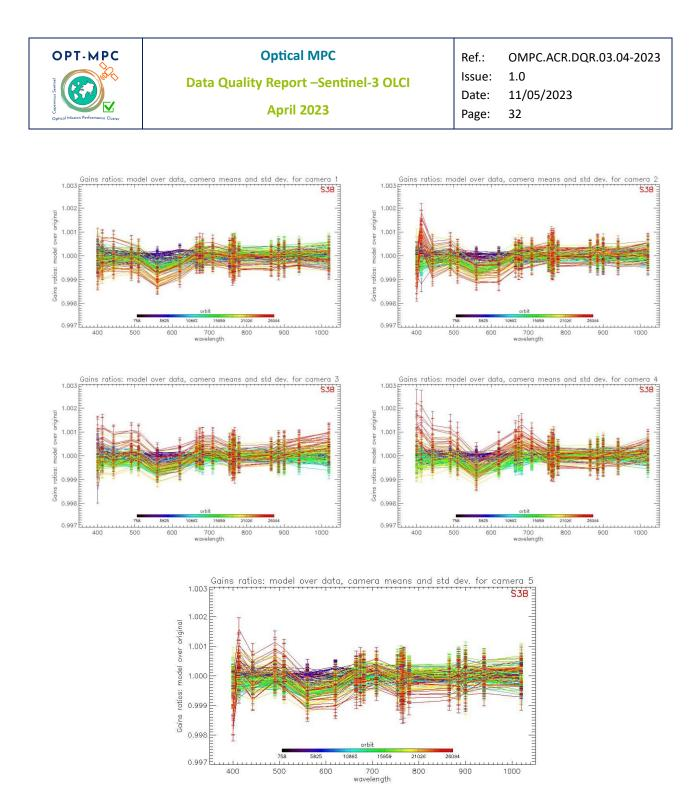
Figure 36: For the 5 cameras: OLCI-B Evolution model performance, as camera-average and standard deviation of ratio of Model over Data vs. wavelength, for each orbit of the test dataset, including 26 calibrations in extrapolation, with a colour code for each calibration from blue (oldest) to red (most recent).
