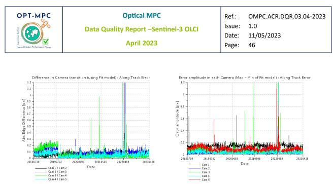
Figure 51: OLCI-A spatial along-track misregistration at each camera transition (left) and maximum amplitude of the along-track error within each camera (left).
