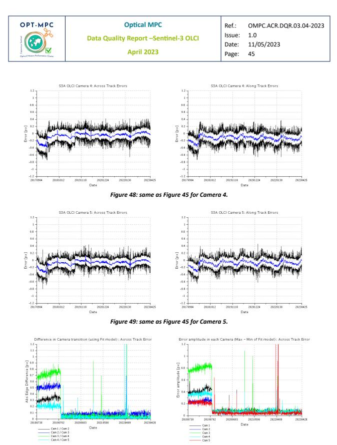
Figure 50: OLCI-A spatial across-track misregistration at each camera transition (left) and maximum amplitude of the across-track error within each camera (left).
