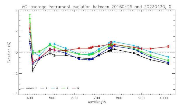
Figure 28: OLCI-A Camera-averaged instrument evolution since channel programming change (25/04/2016) and up to the most recent calibration (30/04/2023) versus wavelength.
