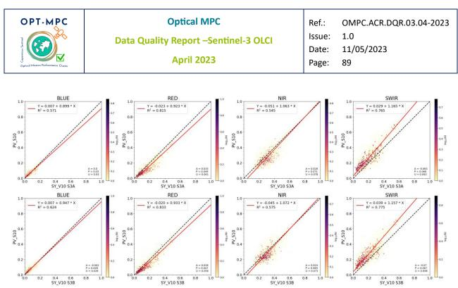
Figure 105: Scatter density plots between SY\_V10 S3A (top) or S3B (bottom) and PROBA-V C2 S10-TOC for BLUE, RED, NIR and SWIR bands (left to right), April/2023 vs. April/2020
