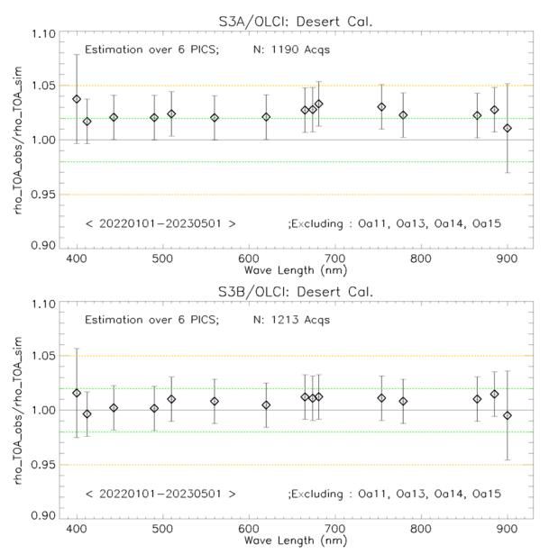
Figure 64: The estimated gain values for OLCI-A and OLCI-B over the 6 PICS sites identified by CEOS over the period January 2022- April 2023 as a function of wavelength. Dashed-green and orange lines indicate the 2% and 5% respectively. Error bars indicate the desert methodology uncertainty.
