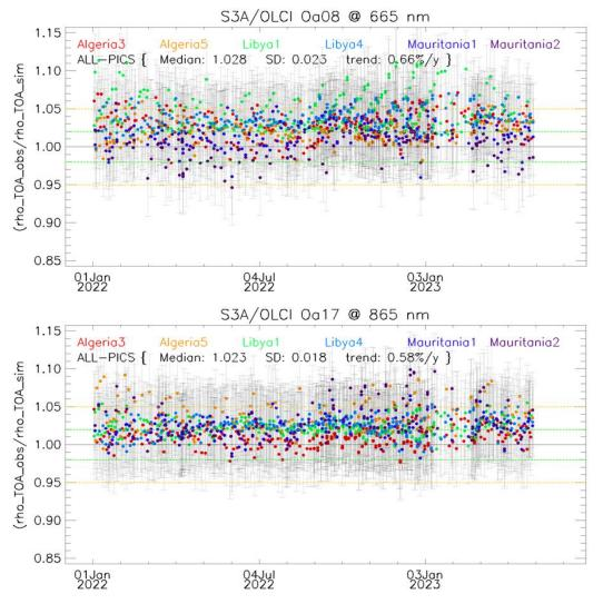
Figure 62: Time-series of the elementary ratios (observed/simulated) signal from OLCI-A for (top to bottom) bands Oa03 and Oa17 respectively over January 2022-April 2023 from the six PICS Cal/Val sites. Dashed-green and orange lines indicate the 2% and 5% respectively. Error bars indicate the desert methodology uncertainty.
