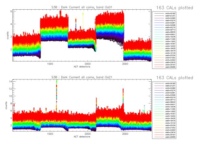
Figure 19: OLCI-B Dark Current for band Oa1 (top) and Oa21 (bottom), all radiometric calibrations so far except the first one (orbit 167) for which the instrument was not thermally stable yet.
