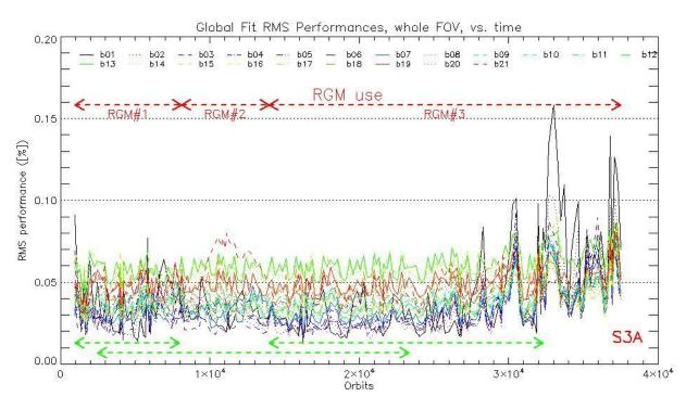
Figure 26: RMS performance of the OLCI-A Gain Model of the current processing baseline as a function of orbit.
