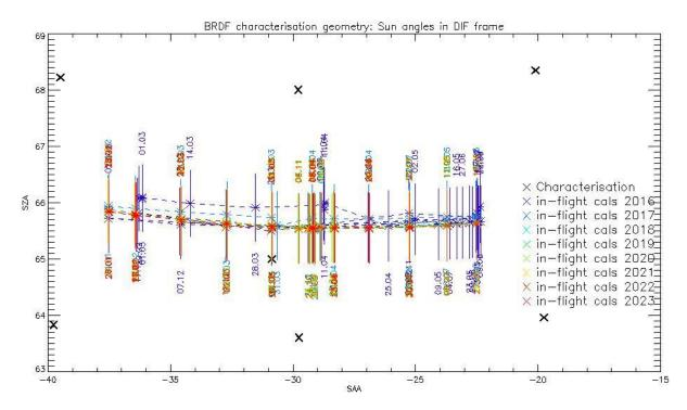
Figure 7: OLCI-A Sun geometry during radiometric Calibrations on top of characterization ones (diffuser frame)
