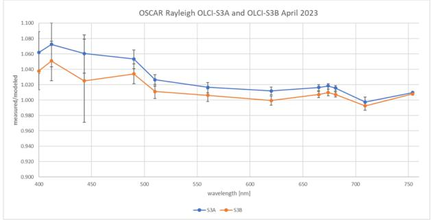
Figure 67: OSCAR Rayleigh S3A and S3B Calibration results as a function of wavelength for April 2023. The results are obtained with a new climatology derived from CMEMS OLCI monthly CHL products.
