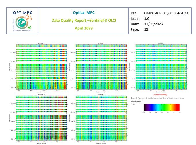
Figure 17: OLCI-B map of periodic noise for the 5 cameras, for band Oa21. X-axis is detector number (East part, from 540 to 740, where the periodic noise occurs), Y-axis is the orbit number. The counts have been corrected from the West detectors mean value (not affected by periodic noise) in order to remove mean level gaps and consequently to have a better visualization of the long term evolution of the periodic noise structure.
