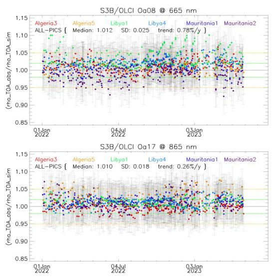
Figure 63: Time-series of the elementary ratios (observed/simulated) signal from OLCI-B for (top to bottom) bands Oa08 and Oa17 respectively over January 2022- April 2023 from the six PICS Cal/Val sites. Dashed-green and orange lines indicate the 2% and 5% respectively. Error bars indicate the desert methodology uncertainty.
