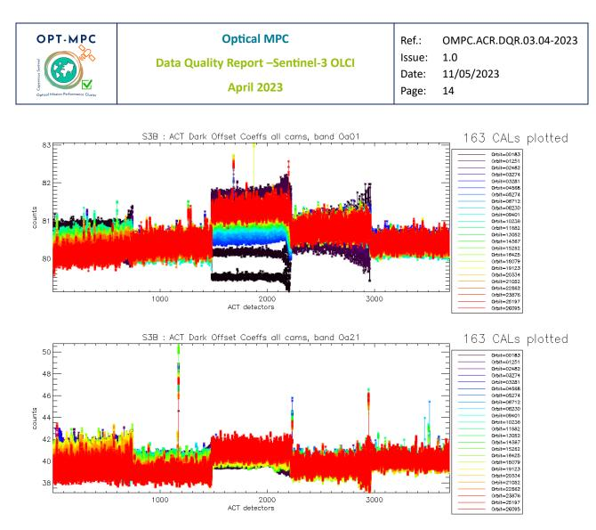
Figure 16: OLCI-B Dark Offset for band Oa1 (top) and Oa21 (bottom), all radiometric calibrations so far except the first one (orbit 167) for which the instrument was not thermally stable yet.
