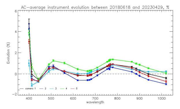
Figure 35: OLCI-B Camera-averaged instrument evolution since channel programming change (18/06/2018) and up to most recent calibration (29/04/2023) versus wavelength.
