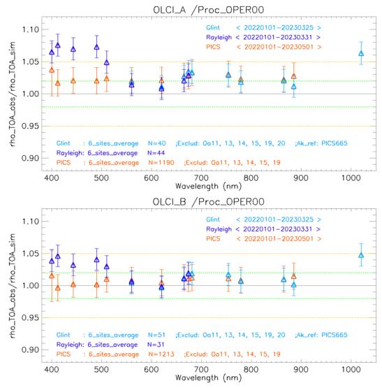
Figure 65: The estimated gain values for OLCI-A and OLCI-B from Glint, Rayleigh and PICS methods over the past twelve months as a function of wavelength. We use the gain value of Oa8 from PICS-Desert method as reference gain for Glint method. Dashed-green and orange lines indicate the 2% and 5% respectively. Error bars indicate the method uncertainties.
