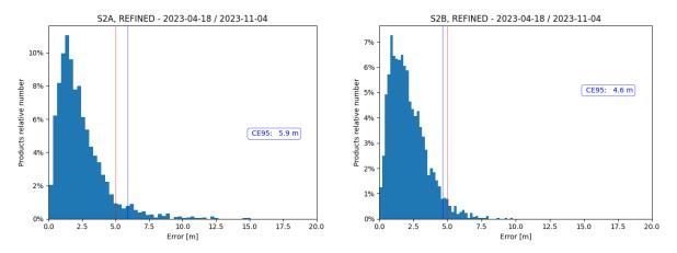
Figure 11: Multi-temporal 2D co-registration errors for refined S2A (left) and S2B pairs (right) (18.04.2023 to 11.04.2023).
