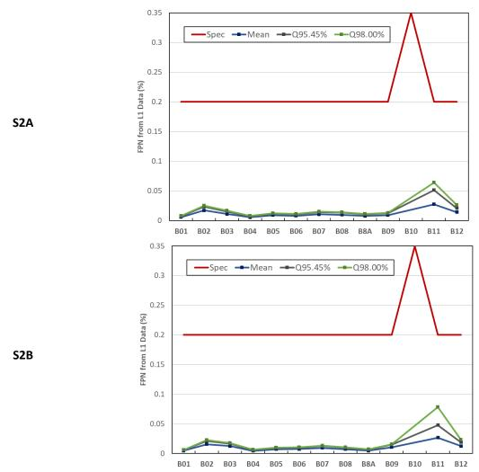
Figure 19 : Fixed Pattern Noise (residual error after equalization) measured on homogeneous natural images for S2A (left) and S2B (right) for Septembre 2023.
