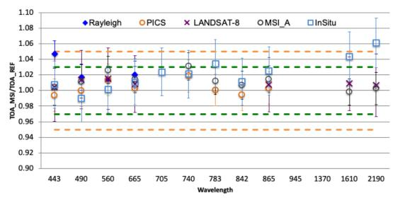
Figure 14: Comparison of radiometric accuracy for all spectral bands (except B09 & B10): ratio of S2B measurement on reference (top) pre-radiometric harmonization between Sentinel-2A and Sentinel-2B in January 2022, (bottom) post-radiometric harmonization up to 10/2023.
