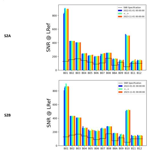
Figure 17: Evolution of the SNR performances based on homogeneous natural acquisitions for S2A (top) and S2B (bottom) from 01/01/2022 to 01/11/2023
