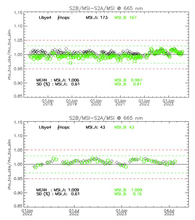
Figure 3: Time-series of the elementary ratios (observed/simulated) signal from MSI-A (black diamonds) and MSI-B (green dots) over the period (top) March 2017 up to August 2023 and (bottom) January 2022 - August 2023 for band B04 from Libya4 PICS Cal/Val site.
