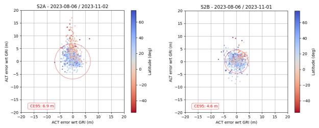
Figure 7: Relative geolocation performance for refined products. Left: S2A, Right: S2B (06.08.2023 – 02.11.2023)
