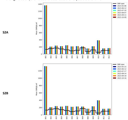
Figure 16: Evolution of the SNR performances based on diffuser acquisitions for S2A from 08/05/2023 to 09/10/2023 (top) and S2B from 15/05/2023 to 16/10/2023 (bottom)
