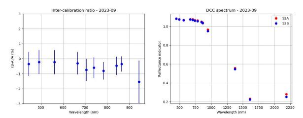
Figure 15: Inter-calibration ratio between S2A and S2B as a function of the wavelength (left) assessed based on acquisitions from September 2023. Reflectance indicator for all wavebands in the VNIR shows an alignment of S2A compared to S2B following the introduction of the radiometric harmonization factor on 01/2022.
