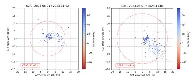
Figure 6: Relative geolocation performance for unrefined products. Left: S2A, Right: S2B (01.05.2023 – 02.11.2023)
