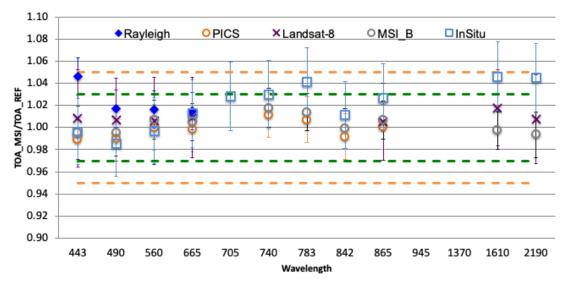
Figure 13: Comparison of radiometric accuracy for all spectral bands (except B09 and B10): ratio of S2A measurement on reference (top) pre-radiometric harmonization between Sentinel-2A and Sentinel-2B in January 2022, (bottom) post-radiometric harmonization up to 10/2023.
