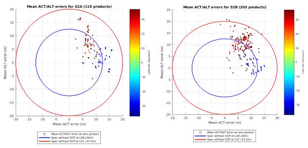
Figure 8: Absolute geolocation performance for unrefined products. Left: S2A, Right: S2B (01.2022 – 09.2023)
