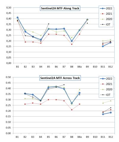
Figure 20 : MTF performance assessments for S2A (along and across track) performed using products from last 3 years and compared to IOT measurements.
