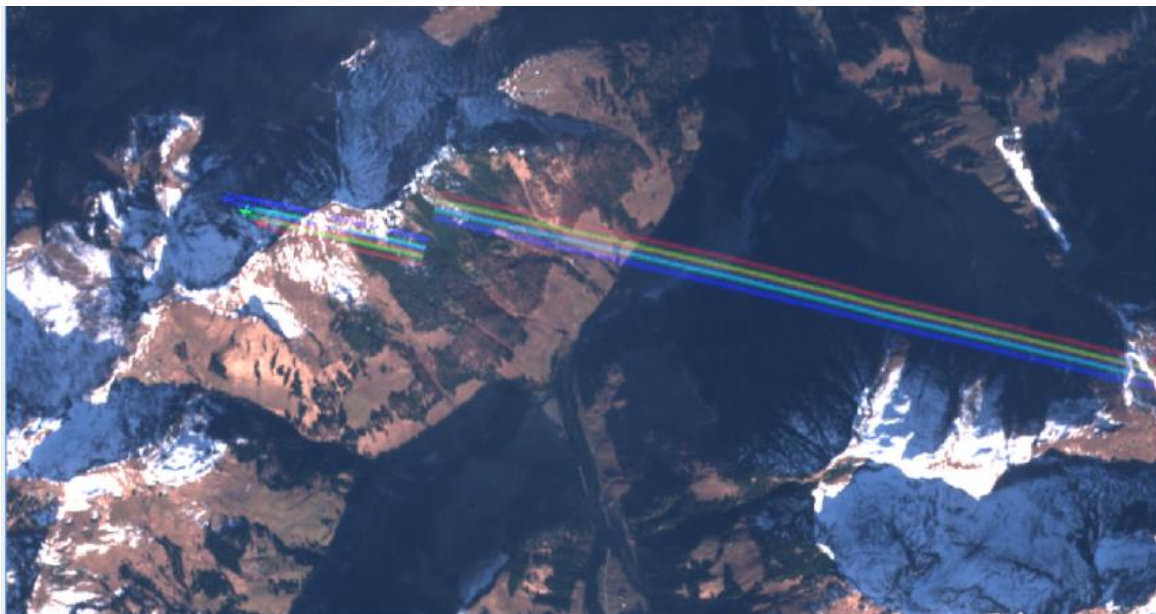
Figure 36: Spectral misregistration and detector misalignment for object at high altitude (plane and contrail). This feature is not an anomaly.
