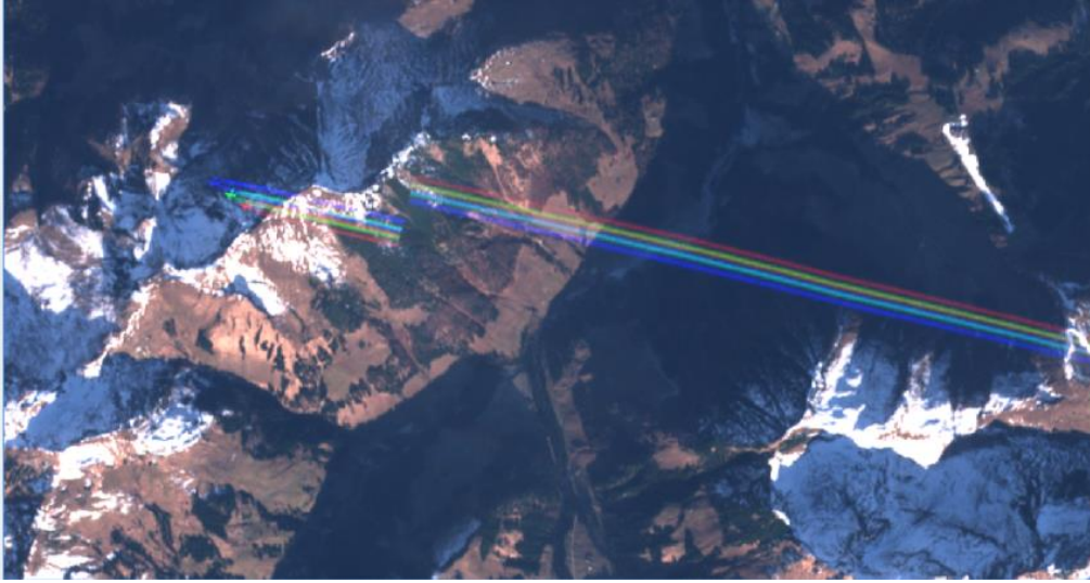
Figure 35: Spectral misregistration and detector misalignment for object at high altitude (plane and contrail). This feature is not an anomaly.
