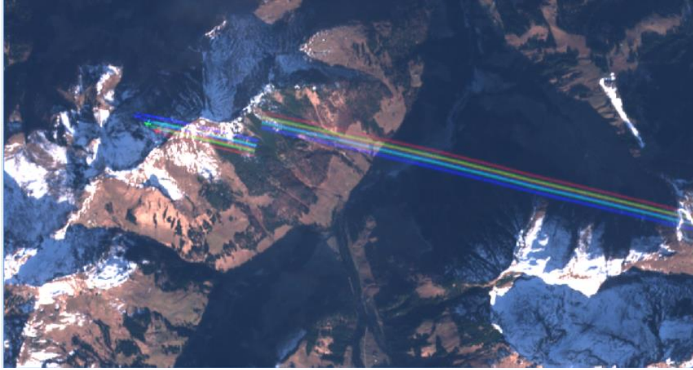
Figure 29: Spectral misregistration and detector misalignment for object at high altitude (plane and contrail). This feature is not an anomaly.
