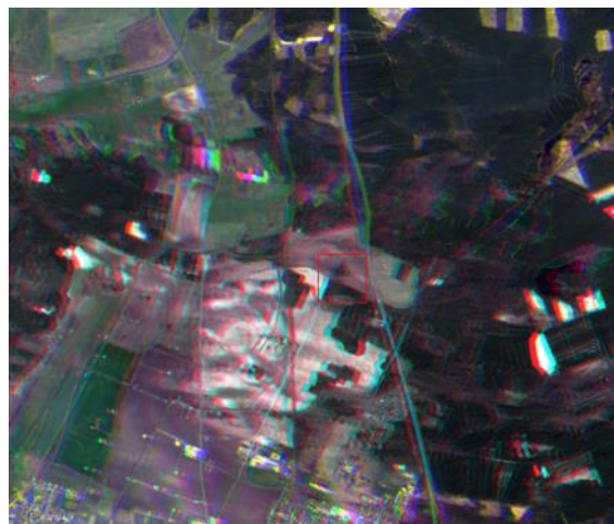
Figure 15: Spectral co-registration error (anomaly #14).
