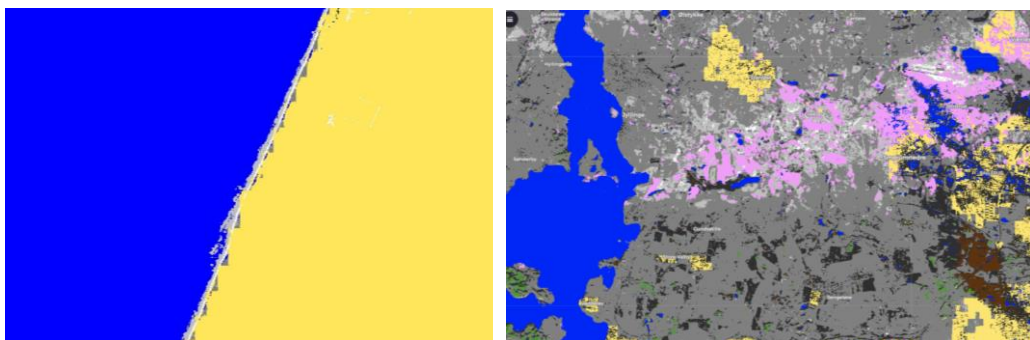
Figure 19: Blocky patterns on the scene classification layer (SCL). Left: near the coastline. Right: near city boundaries.
