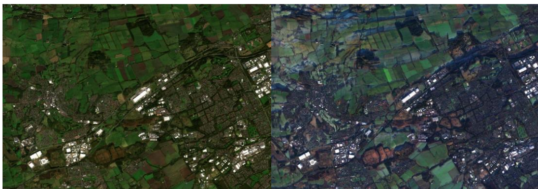
Figure 21: L2A True Colour Image of tile 30VVH; left: 10/10/2018, SZA = 62°; right: 24/12/2018, SZA = 80°. The radiometric quality for surface reflectance is not ensured for SZA > 70°.
