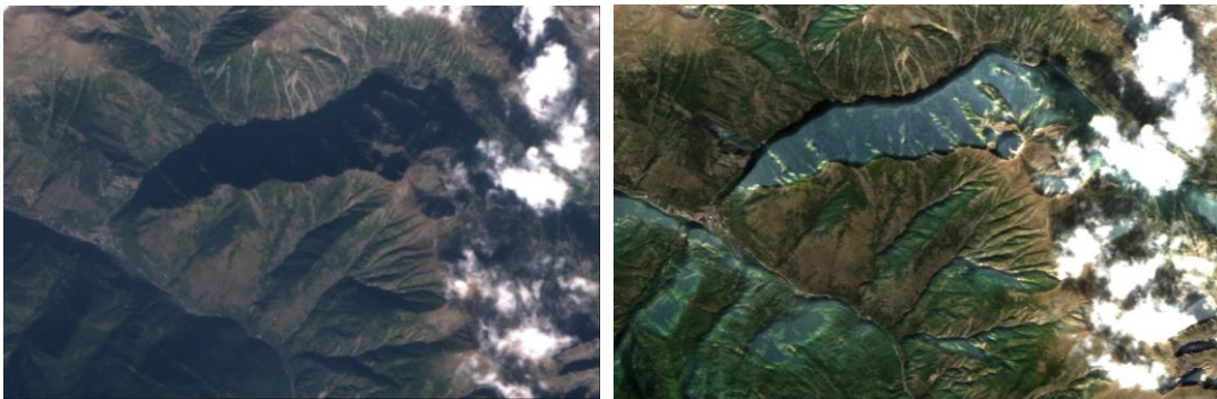
Figure 20: Terrain over-correction on shaded areas. Left: Level 1C true colour image, right: L2A true colour image.
