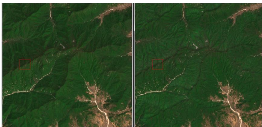
Figure 13: Left: affected product processed without DEM. Right: corrected product processed with DEM (anomaly #7).
