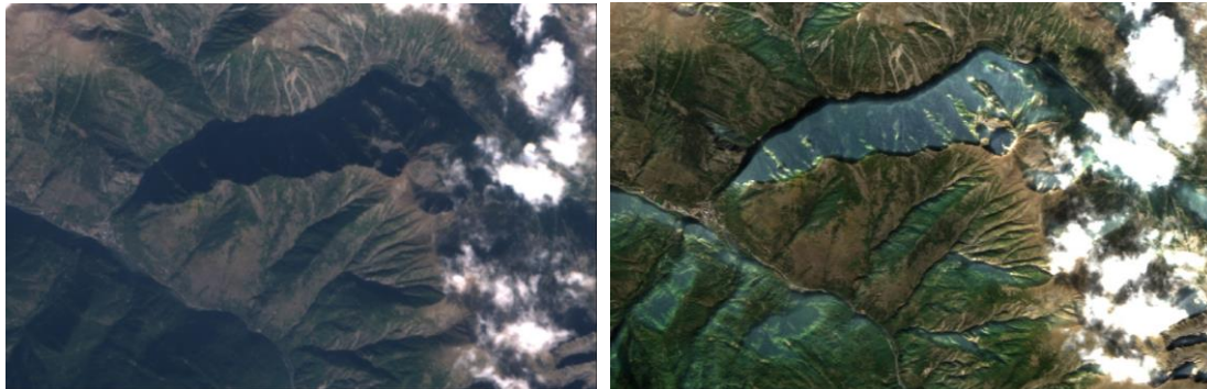
Figure 20: Terrain over-correction on shaded areas. Left: Level 1C true colour image, right: L2A true colour image.
