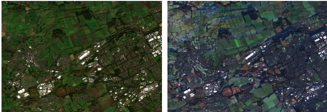
Figure 15: L2A True Colour Image of tile 30VVH; left: 10/10/2018, SZA = 62°; right: 24/12/2018, SZA = 80°. The radiometric quality for surface reflectance is not ensured for SZA > 70°.
