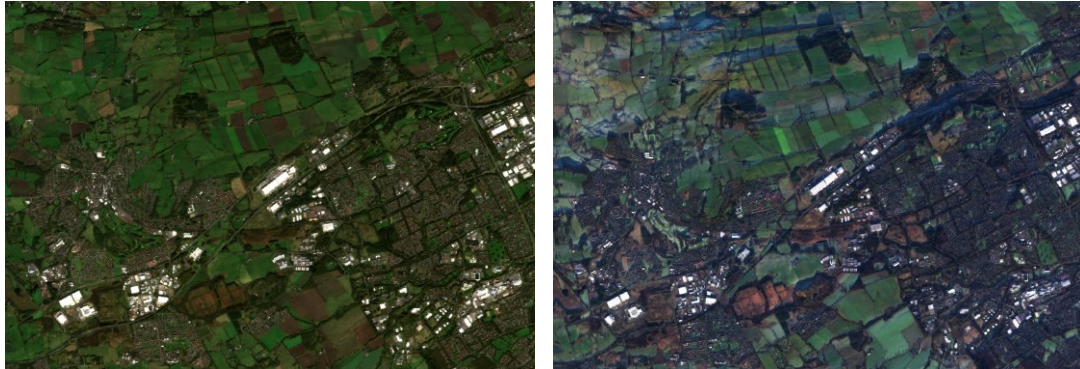
Figure 14: L2A True Colour Image of tile 30VVH; left: 10/10/2018, SZA = 62^\circ ; right: 24/12/2018, SZA = 80^\circ . The radiometric quality for surface reflectance is not ensured for SZA > 70^\circ .
