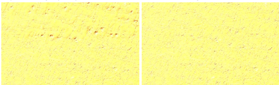
Figure 7: 10 m True Color Images of tiles 32RLV and 32LRU acquired on 14/04/2019. Left: processing baseline 02.11 – terrain correction is not applied on tile 32RLV which leads to a visual discontinuity in the image. Right: processing baseline 02.12 – terrain correction is applied on both tiles and no discontinuity can be seen.
