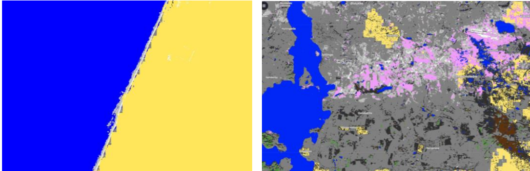
Figure 12: Blocky patterns on the scene classification layer (SCL). Left: near the coastline. Right: near city boundaries.
