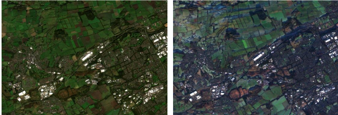
Figure 13: L2A True Colour Image of tile 30VVH; left: 10/10/2018, SZA = 62°; right: 24/12/2018, SZA = 80°. The radiometric quality for surface reflectance is not ensured for SZA > 70°.
