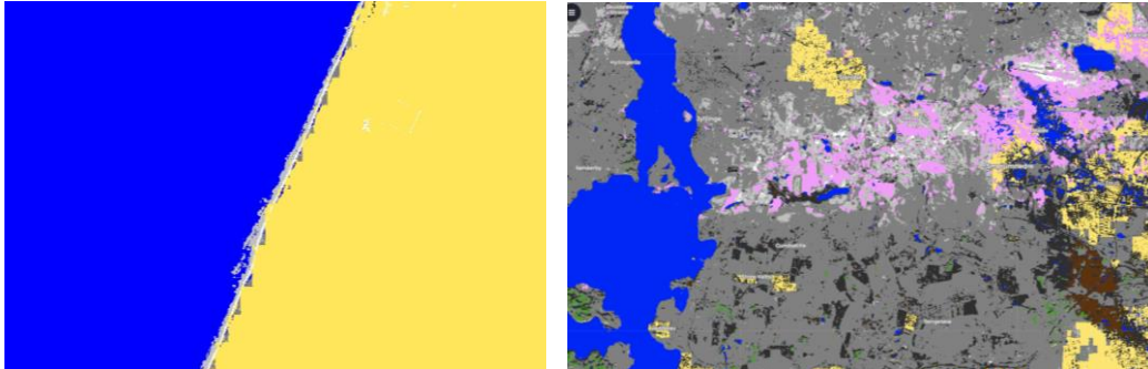
Figure 11: Blocky patterns on the scene classification layer (SCL). Left: near the coastline. Right: near city boundaries.
