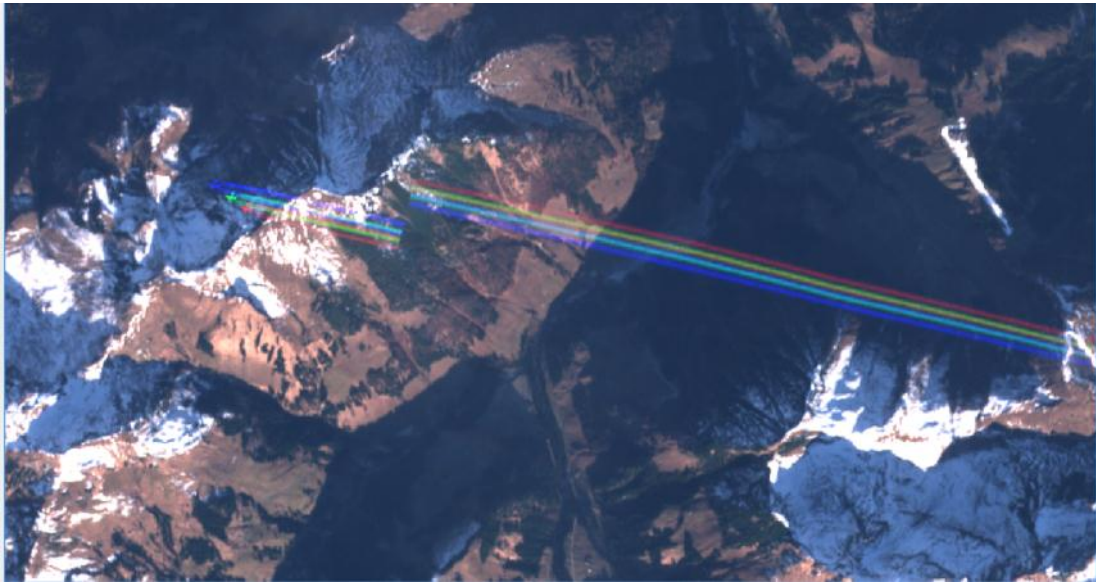
Figure 15: Spectral misregistration and detector misalignment for object at high altitude (plane and contrail). This feature is not an anomaly.
