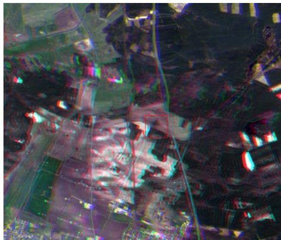
Figure 12: Spectral co-registration error (anomaly #14).
