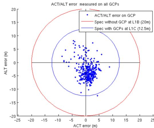
**Figure 1: Geolocation performance measured on 44 products since 15/11/2106 (for all Ground Control Points in Across-Track/Along-Track frame).**
