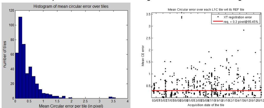
**Figure 2: Histogram (left) and Time series (right) of the multi-temporal performance. The 3 m requirement will be applicable only after activation of the geometrical refinement. The current performance is 12 m at 95% confidence.**
