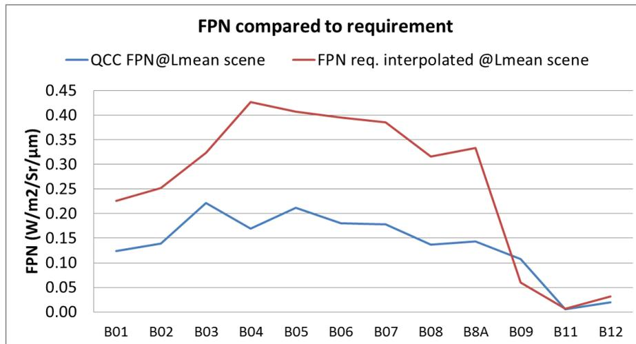
**Figure 6: Measured Fixed Pattern Noise (residual error after equalization) on quasi-uniform scenes (blue curve), compared to requirement interpolated at scene radiance (red curve). The noise is better than requirements for VNIR bands and close to requirements for SWIR bands.**
