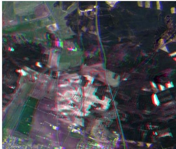
**Figure 12: Spectral co-registration error (anomaly #14).**
