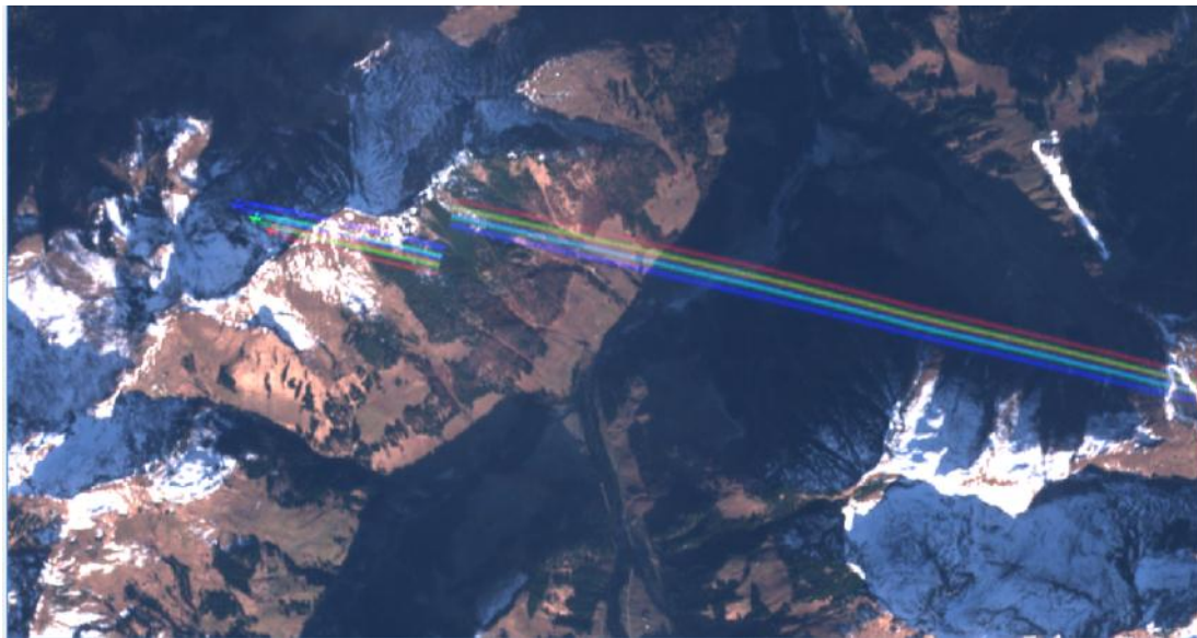
Figure 19: Spectral misregistration and detector misalignment for object at high altitude (plane and contrail). This feature is not an anomaly.
