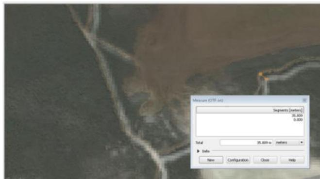
**Figure 17: S2 image superimposed with reference map, showing a geolocation error of 35 m (anomaly #18).**
