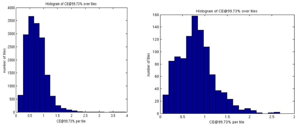
**Figure 2: Histogram of the multi-temporal performance for S2A (left) and S2B (right, different scale). The 3 m requirement will be applicable only after activation of the geometrical refinement. The current performance is 11 m (S2A) and 14 m (S2B) at 95% confidence.**
