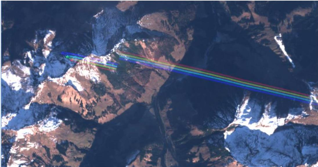
**Figure 21: Spectral misregistration and detector misalignment for object at high altitude (plane and contrail). This feature is not an anomaly.**
