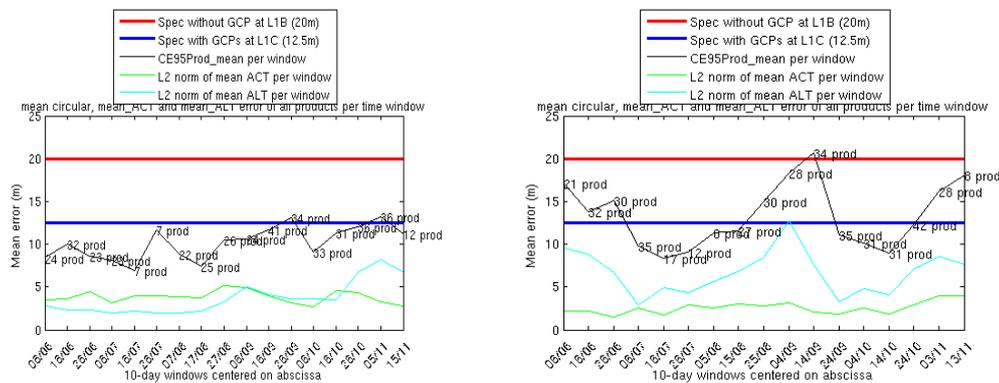
**Figure 1: Geolocation performance for S2A (left) and S2B (right). The performance is computed over a sliding window of 30 (respectively 10) days for S2A (resp. S2B). The vertical dashed lines for S2B indicate the calibration updates. (ACT= across track, ALT = along track)**
