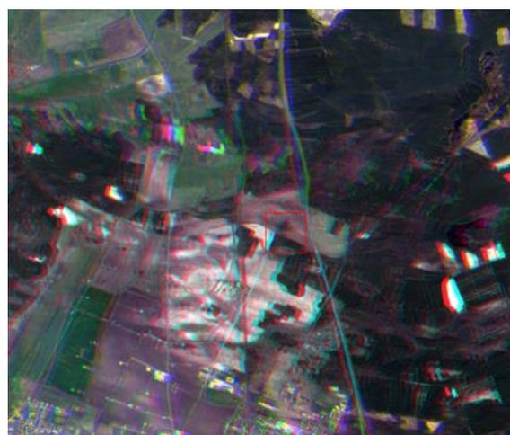
**Figure 14: Spectral co-registration error (anomaly #14).**
