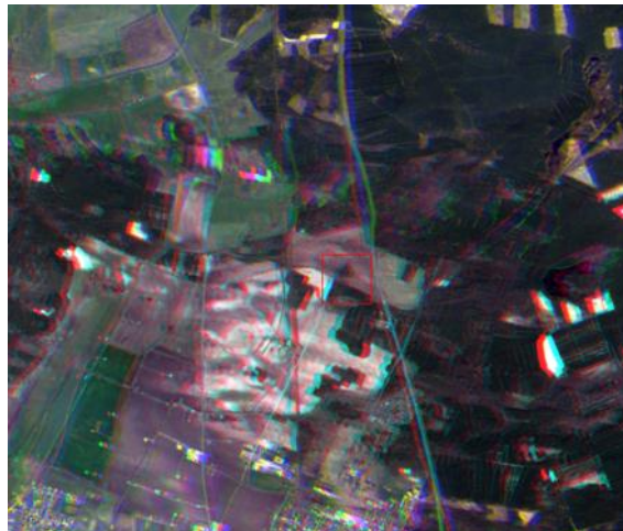
Figure 12: Spectral co-registration error (anomaly #14).
