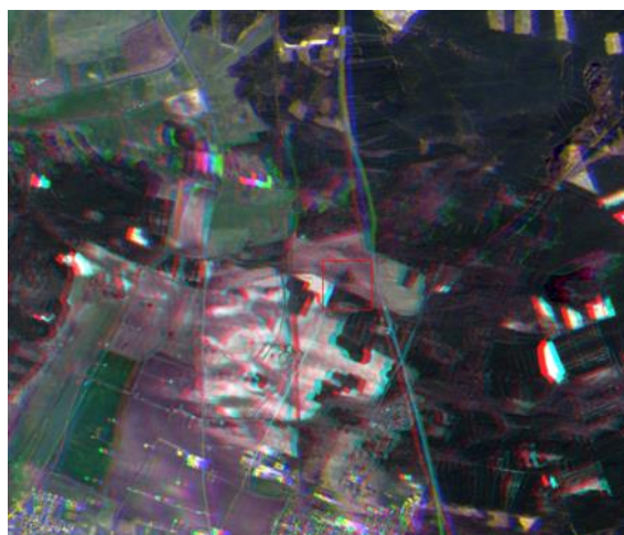
Figure 14: Spectral co-registration error (anomaly #14).
