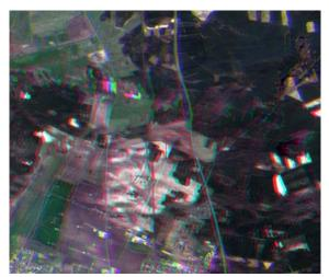
Figure 14: Spectral co-registration error (anomaly #14).
