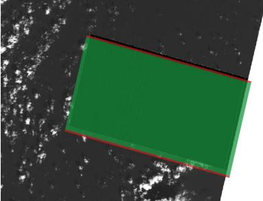
Figure 18: Technical Quality masks (green: lost packets, red: degraded packets) overlayed over an affected imaged. A small gap exists between the mask and the affected area (anomaly #21).
