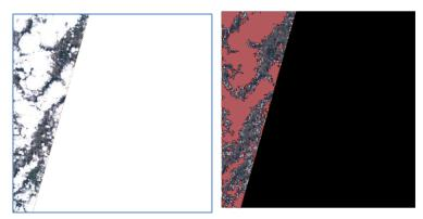
Figure 20: Tile 40UGE acquired on 12/06/2018 by S2B. Left: RGB composite, Right: cloud mask (in red). The cloud coverage percentage is incorrectly reported as 19.3% (anomaly #44).
