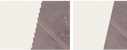
Figure 7: Swath boundary with the current processing baseline 02.06 (Left) and new processing baseline 02.07 (Right). The coarse staircaselike boundary has been refined. More valid pixels are provided.
