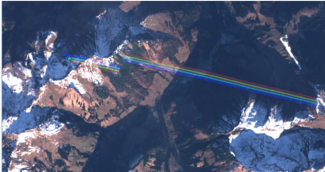
Figure 27: Spectral misregistration and detector misalignment for object at high altitude (plane and contrail). This feature is not an anomaly.
