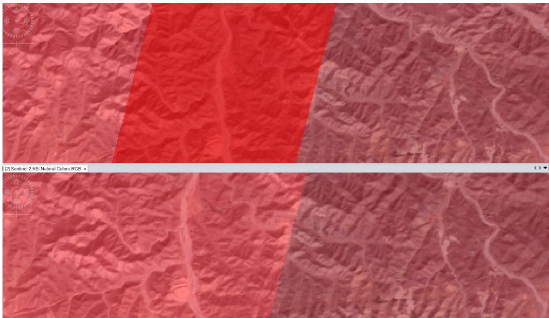
Figure 8: Detector footprints for the current processing baseline 02.06 (top) and new processing baseline 02.07 (bottom). The detector footprint do no longer include the overlap area.
