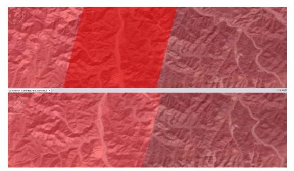
Figure 8: Detector footprints for the current processing baseline 02.06 (top) and new processing baseline 02.07 (bottom). The detector footprint no longer includes the overlap area.
