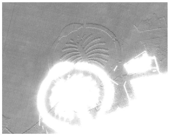
Figure 28: Gradient cross-talk on band B12 (highly enhanced contrast).
