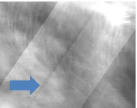
Figure 24: Along-track stripe on B11 image due to a non-linear response on D11 (contrast strongly enhanced).
