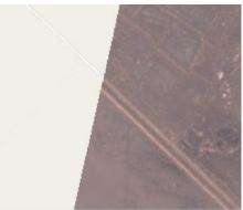
Figure 7: Swath boundary with the current processing baseline 02.06 (Left) and new processing baseline 02.07 (Right). The coarse staircaselike boundary has been refined. More valid pixels are provided.
