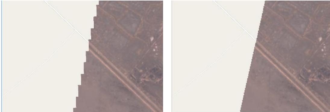
**Figure 7: Swath boundary with the current processing baseline 02.06 (Left) and new processing baseline 02.07 (Right). The coarse staircase-like boundary has been refined. More valid pixels are provided.**
