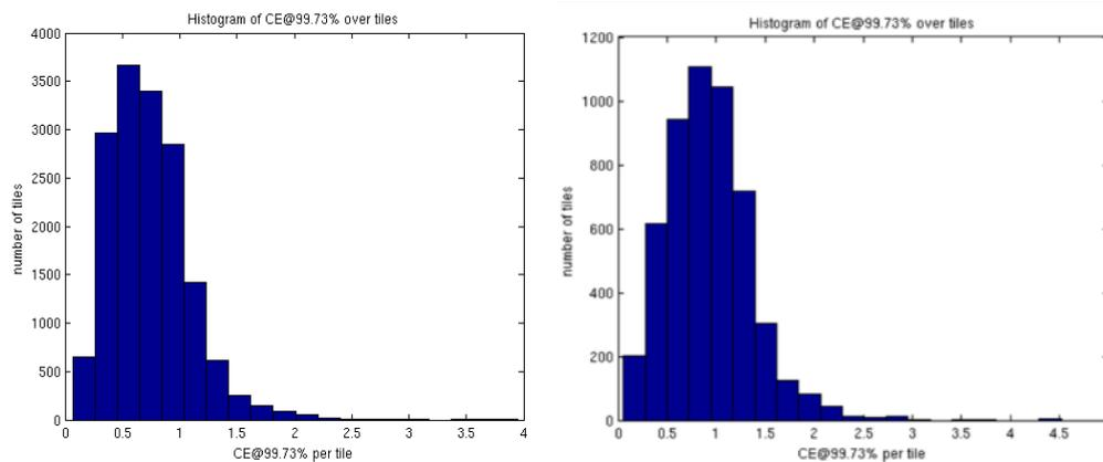
**Figure 2: Histogram of the multi-temporal performance for S2A (left) and S2B (right, different scale). The 3 m requirement will be applicable only after activation of the geometrical refinement. The current performance is 11 m (S2A) and 13 m (S2B) at 95% confidence.**
