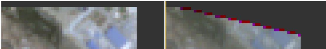
**Figure 23: Top-right corner of the image of the same L1C tile from orbit 7053 (unaffected, left) and orbit 7196 (affected, right). (Anomaly #46)**
