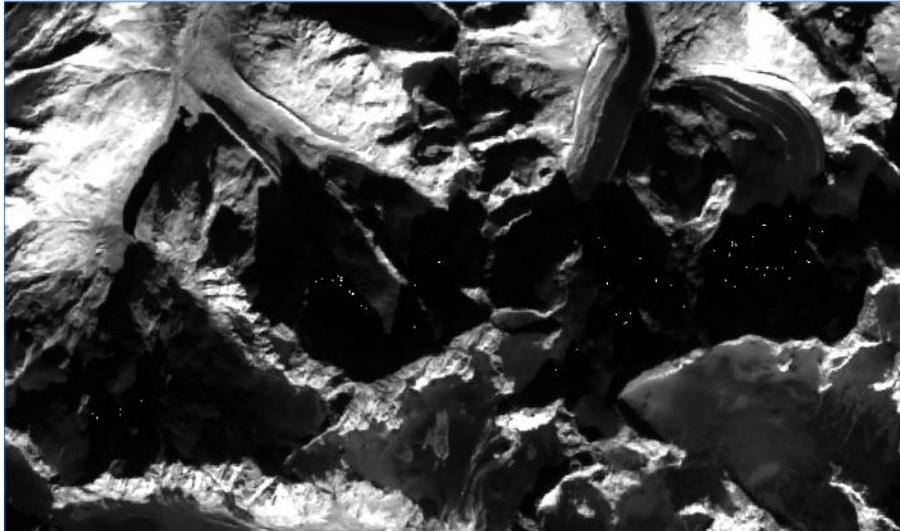
**Figure 21: Pixels with 0 value (No Data) shown here as transparent, in a dark area of a B12 image (Anomaly #5).**
