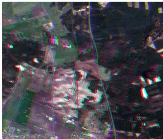
**Figure 14: Spectral co-registration error (anomaly #14).**
