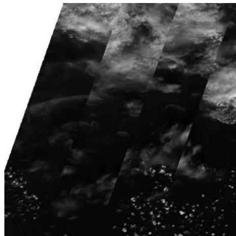
**Figure 16: Detector misalignment on band B1 (anomaly #17).**
