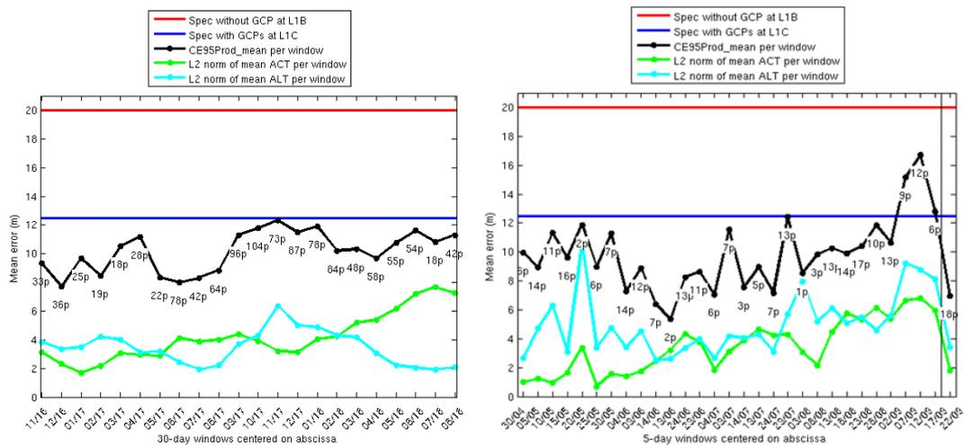
**Figure 1: Geolocation performance for S2A (left) and S2B (right). The performance is computed over a sliding window of 30 days (S2A, left) or 5 days (S2B, right). Number of products used in the sliding window indicated for each point. (ACT= across track, ALT = along track). A vertical line indicates a geometric calibration event.**
