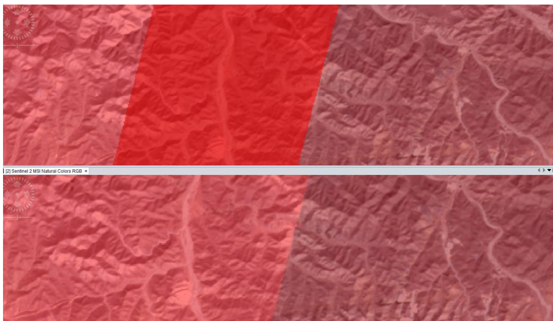
Figure 9: Detector footprints for the current processing baseline 02.06 (top) and new processing baseline 02.07 (bottom). The detector footprint do no longer include the overlap area.
