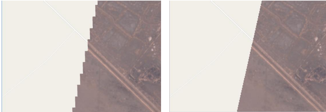
Figure 8: Swath boundary with the current processing baseline 02.06 (Left) and new processing baseline 02.07 (Right). The coarse staircase-like boundary has been refined. More valid pixels are provided.
