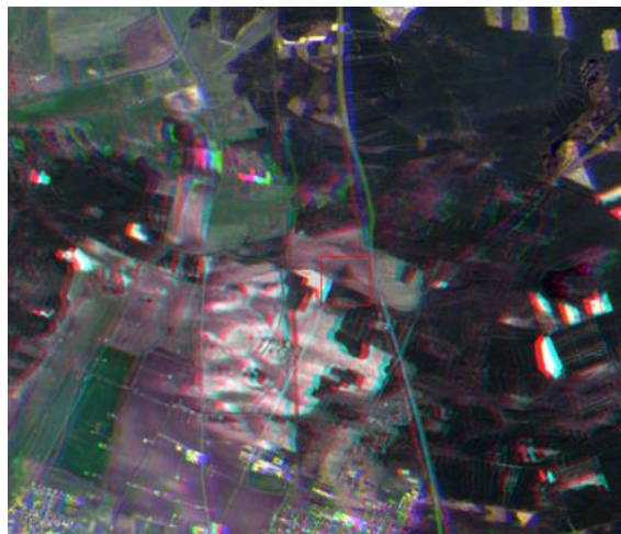
Figure 15: Spectral co-registration error (anomaly #14).
