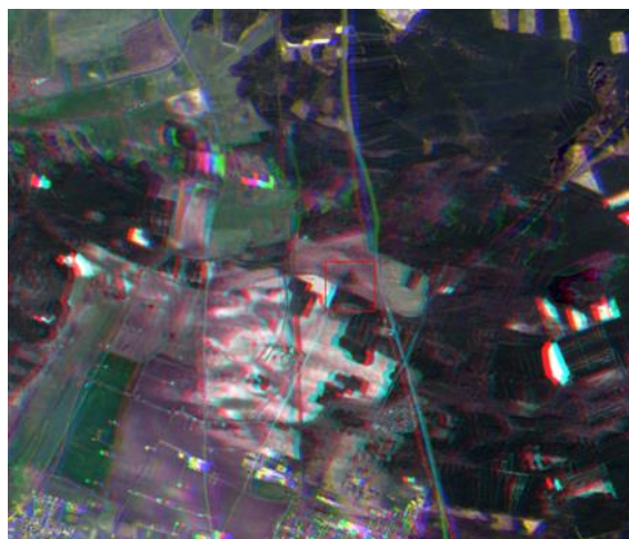
Figure 12: Spectral co-registration error (anomaly #14).
