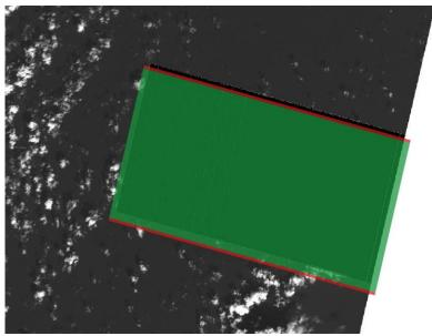
Figure 16: Technical Quality masks (green: lost packets, red: degraded packets) overlayed over an affected imaged. A small gap exists between the mask and the affected area (anomaly #21).
