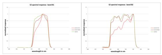
Figure 3: Spectral Response Functions for bands B01 and B02. Red – dashed: S2A before correction. Red – solid: S2A after correction. Green: S2B.
