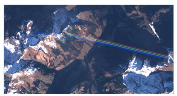
Figure 19: Spectral misregistration and detector misalignment for object at high altitude (plane and contrail). This feature is not an anomaly.
