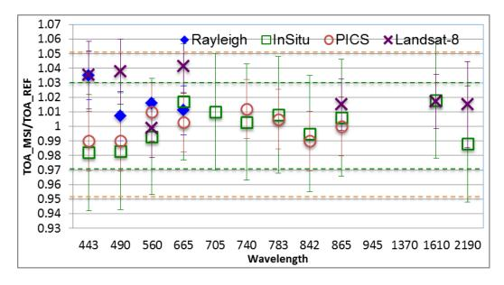
Figure 4: Comparison of radiometric accuracy for all spectral bands (except B10 and B09): ratio of S2A measurement on reference. Error bars indicate the method uncertainty.
