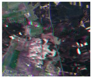
Figure 12: Spectral co-registration error (anomaly #14).
