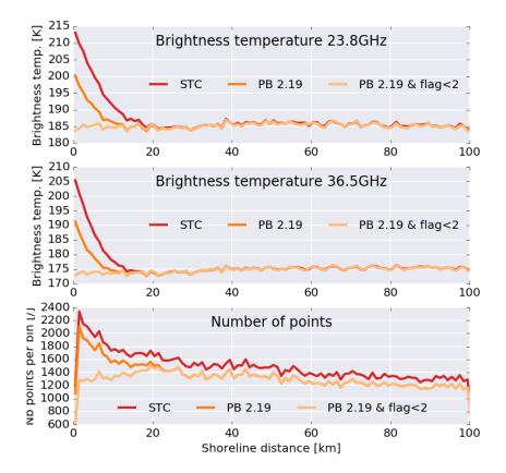
Figure 6: Interpolated brightness temperature as a function to the shoreline distance for previous processing baseline (red) and Processing Baseline 2.24 (orange). The light orange curve shows the result when selecting configuration with along track averaging flag <2 (nominal or extrapolated), the interpolated brightness temperature is no longer impacted by the land contamination, but the number of points is reduced.
