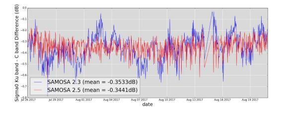
Figure 1 Mean per pass of the difference between SARM Ku band and C band backscatter coefficient for previous processing baseline (blue curve) and Processing Baseline 2.24 (red curve)
