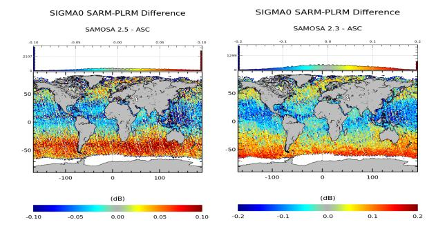
Figure 4 Difference between SARM Ku band and PLRM Ku band backscatter coefficient for previous processing baseline (right map) and Processing Baseline 2.24 (left map). The maps display only the ascending tracks to better highlight the finer details of the difference in the maps.
