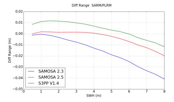
Figure 2 Difference between SARM Ku band and PLRM Ku band range wrt SWH for previous processing baseline (blue curve) and Processing Baseline 2.24 (green curve). The curve obtained for the CNES S3 prototype (red curve) is also represented to provide an external reference.
