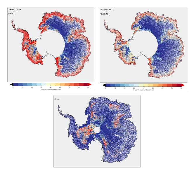
Figure 9 Percentage of failure over Antarctica of the ice sheet retracker with previous processing baseline (upper left) and Processing Baseline 2.24 (upper right). The percentage of failure with Cryosat-2 mission is also displayed for comparison (bottom). Note that the margins are acquired in SARin mode on Cryosat-2 mission, which explains the very low percentage of failure over this zone.
