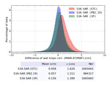
Figure 5 Difference between 5 parameters radiometer and ECMWF model wet tropospheric correction for previous processing baseline (red) and Processing Baseline 2.24 (blue). The results obtained for the 3 parameter correction is also provided (green histogram)
