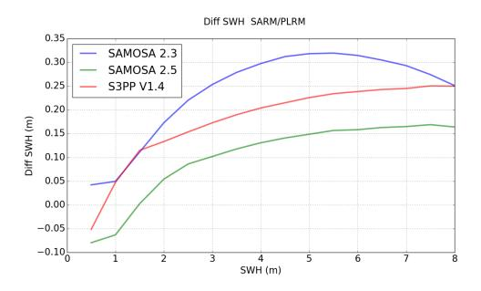
Figure 3 Difference between SARM Ku band and PLRM Ku band SWH wrt SWH for previous processing baseline (blue curve) and Processing Baseline 2.24 (green curve). The curve obtained for the CNES S3 prototype (red curve) is also represented to provide an external reference.
